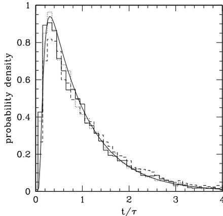
FIG. 4. Probability density of translocation times for one-dimensional phantom polymers. Solid, dotted and dashed lines correspond to polymer lengths  $N = 32, 64$  and  $128$ , respectively, and were extracted from 10,000 simulations, each. The times have been normalized by their respective mean translocation time  $\tau(N)$  in each case. The continuous curve corresponds to the solution of the Fokker-Planck equation in the single-particle approximation.
