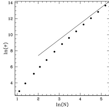
FIG. 5. Logarithmic plot of the mean translocation time  $\tau$  as a function of chain length  $N$  for a one dimensional phantom polymer. Each data point represents an average over 10,000 realizations. The solid line has slope 2.
