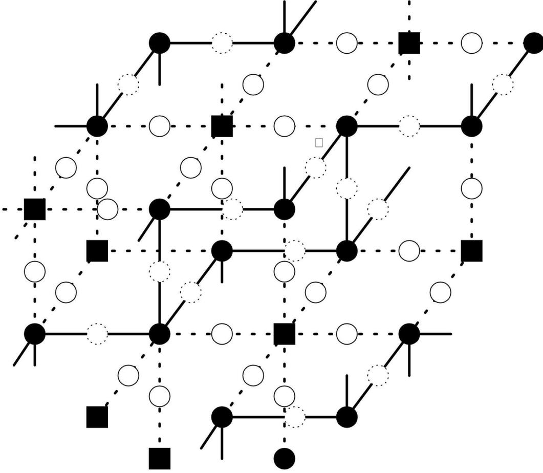
FIG. 4. Ordering of  $Mn^{3+}$  ions (black circles),  $Mn^{4+}$  ions (black squares),  $1e - \sigma$  bonds formed by singlet pairs (dashed lines), and  $1e - \sigma^*$  bonds formed by triplet pairs (solid lines) in  $A_{0.67}B_{0.33}MnO_3$ . Dashed open circles show  $O^{2-}$  ions in the  $3s2p$  hybrid state. Local distortions are not shown.
