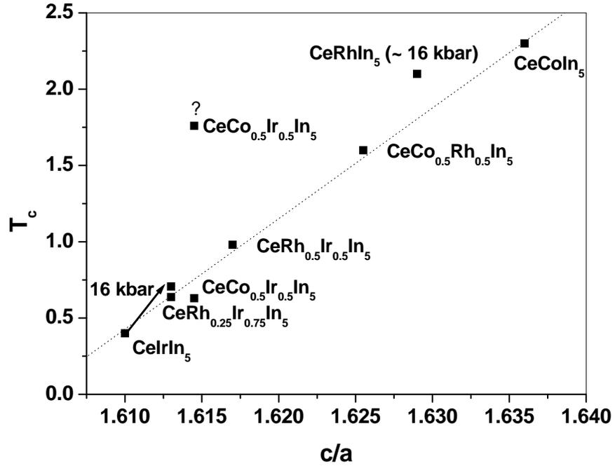
FIG. 2.  $T_c$  as a function of  $c/a$  for the  $\text{Ce}(\text{Rh},\text{Ir},\text{Co})\text{In}_5$  HFS.
