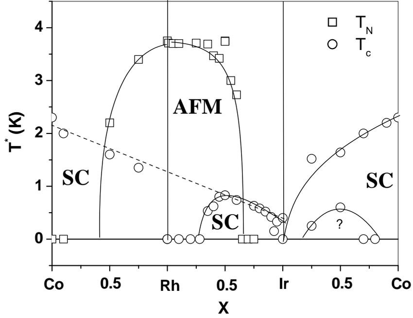
FIG. 1. Phase Diagram of  $\text{Ce}(\text{Rh},\text{Ir},\text{Co})\text{In}_5$
