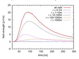
Fig. 26. Contribution of different lateral rings to the radio pulse at 75 m north from the shower centre.
