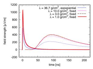
Fig. 13. Radio signal convergence in a fully histogrammed air shower when going from 36.7 g cm<sup>-2</sup>, exponentially distributed, to 1.0 g cm<sup>-2</sup>, fixed track lengths.
