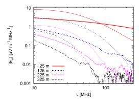
Fig. 18. Overall change in the radio signal frequency spectra between REAS1 (thin lines) and REAS2 (thick lines) at various distances to the north of the shower centre.
