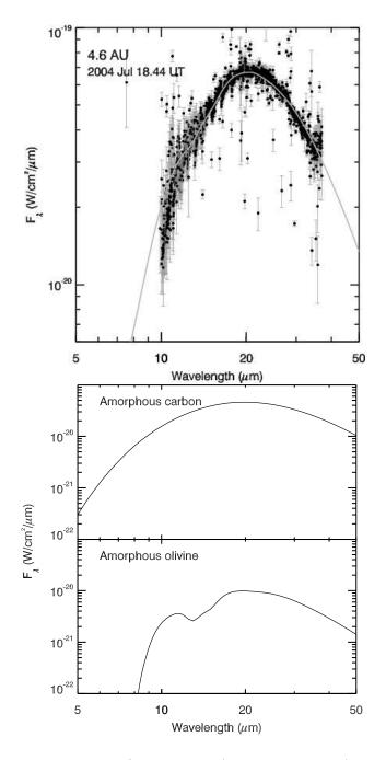
Fig. 13.— IRS spectrum of comet C/2001 HT50 (LINEAR-NEAT) at r = 4.6 AU and bestfit model of the dust thermal emission (N = 3.7, M = 29.6,  $a_p = 1.2 \ \mu m$ ). Also shown are the decomposed spectra for each of the significant minerals in the best-fit model.
