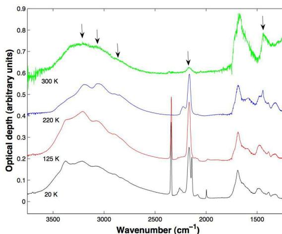
**Fig. 3.** Comparison of the spectra of (from the bottom to the top): formamide after irradiation with a dose of 24 eV/16amu at 20 K, and after warming up at 125 K, 220 K and room temperature (this spectrum was magnified 5 times). The arrows show the bands corresponding to the presence of  $NH_4^+OCN^-$ . Spectra have been arbitrarily shifted for sake of clarity.
