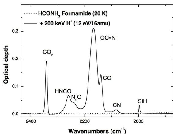
**Fig. 2.** IR transmittance spectrum in optical depth scale of formamide (20 K) after irradiation at a dose of 12 eV/16amu with 200 keV  $H^+$  ions (full line). The spectrum obtained before irradiation is also shown (dotted line).
