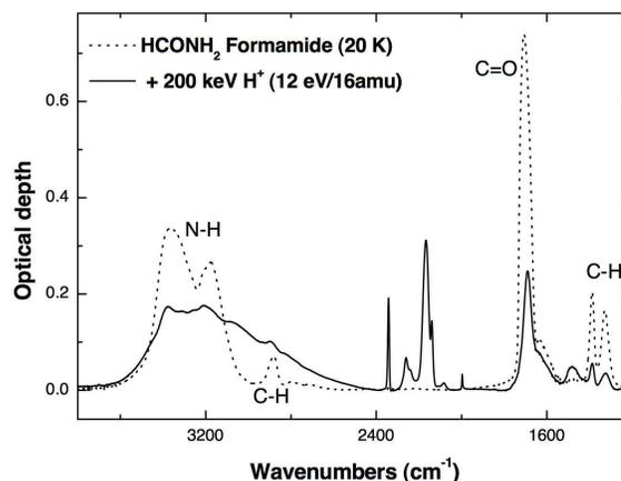
**Fig. 1.** IR transmittance spectrum in optical depth scale of formamide as deposited at 20 K on a silicon substrate (dot line). The band–peak positions and assignment are given in Table 1. The spectrum obtained after irradiation at a dose of 12 eV/16amu with 200 keV H<sup>+</sup> ions is also shown (full line).
