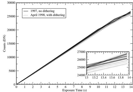
FIG. 3.— Comparing non-destructive readouts from dithered and un-dithered data for CHA-DC-F7. Inset: An expanded view from the end of the exposures highlighting the photometric differences.
