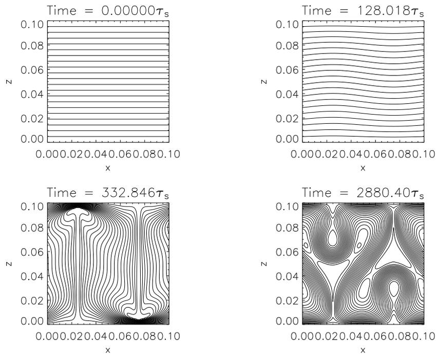
Fig. 4.— Snapshots of the magnetic field lines in run N1 at various times during the evolution of the instability. (upper left) Initial condition; (upper right) Linear phase; (lower left) Non-linear phase; (lower right) Saturated state.
