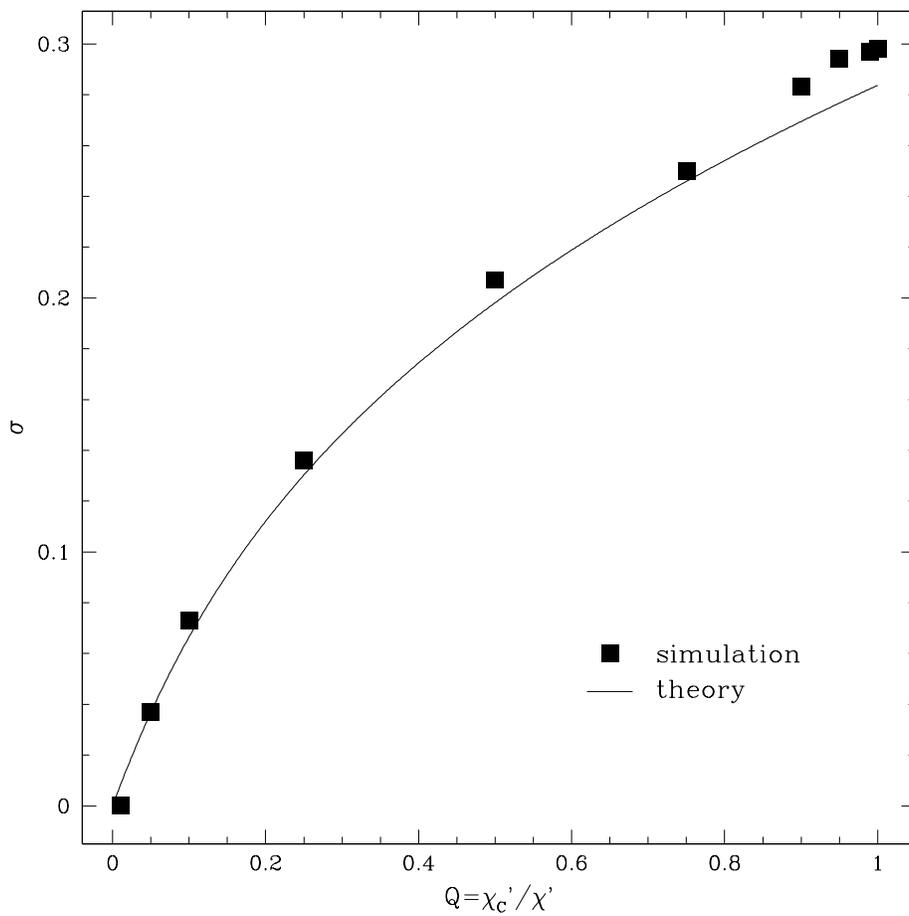
Fig. 3.— The effect of isotropic conductivity. Holding the total conductivity  $\chi_{\text{tot}}$  and all other quantities fixed, the anisotropic fraction,  $Q$ , is varied. As  $Q$  approaches 1.0, conduction is purely anisotropic, and the growth rate reaches an asymptotic value. As the conduction becomes more isotropic, *i.e.*  $Q$  approaches zero, the instability is quenched. The solid line marked 'theory' is the unstable branch in the solutions of equation 16
