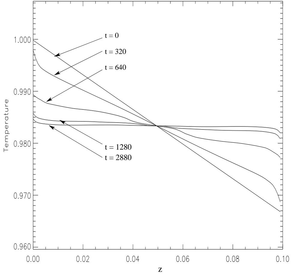
Fig. 6.— Vertical profile of the horizontally-averaged temperature profile in run N1 at various times. The initial state is a monotonically decreasing temperature profile with respect to height, and the final state is isothermal.
