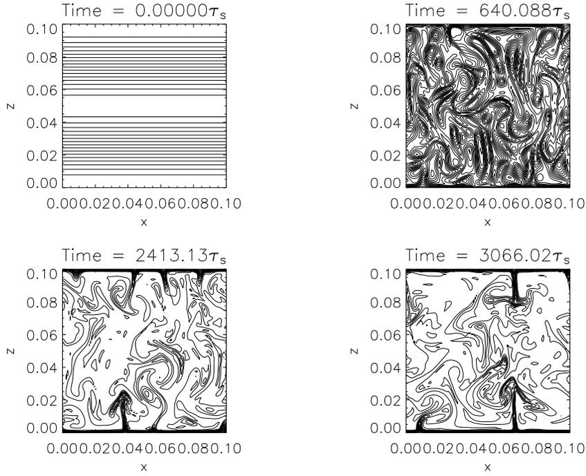
Fig. 10.— Snapshots of the magnetic field lines at various times during the evolution of run N3. (upper left) The initial magnetic field. (upper right) Early non-linear growth is marked by highly complex field geometry, reconnection, and generation of vorticity. The bottom plots show narrow plumes generated at the boundaries. A thermal boundary layer is evident at the upper and lower surfaces.
