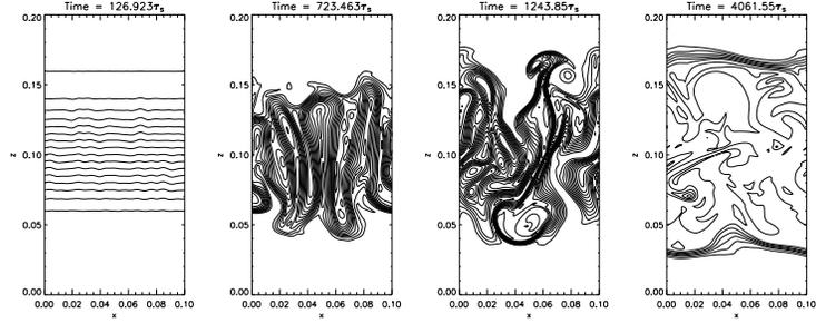
Fig. 15.— Snapshots of the magnetic field in Run N4. (far left) Early linear phase; (middle left) early non-linear phase. (middle right) The MTI drives penetrative convection into the stable layers, and at late times (far right) magnetic flux is pumped into the stable layers.
