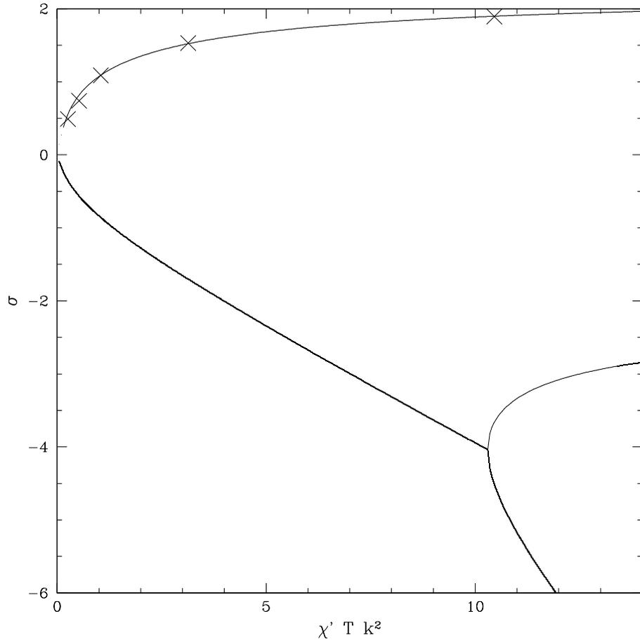
Fig. 1.— Solutions of the MTI dispersion relation in the weak field limit for an atmosphere with  $d \ln T / d \ln S = -3$ . The axes are normalized to the local Brunt-Väisälä frequency,  $N$ . The crosses are growth rates measured from simulations (see §3.1).
