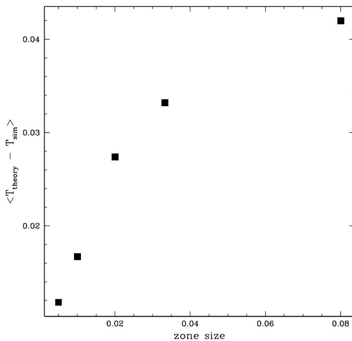
Fig. 17.— The convergence of the average error with resolution for the circular conduction test problem.
