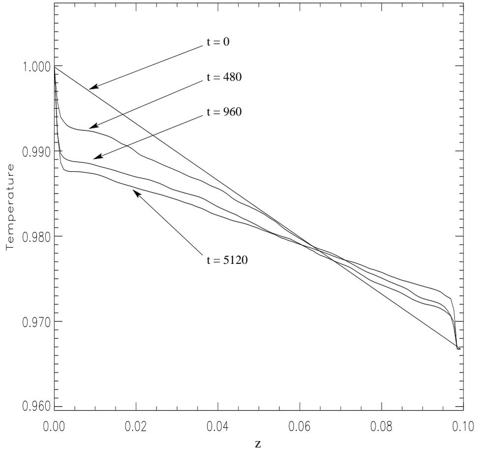
Fig. 12.— Vertical profiles of the horizontally averaged temperature at various times in Run N3. A narrow thermal boundary layer develops, while the interior saturates to a more isothermal profile than the initial state. The width of the boundary layers is resolution-dependent.
