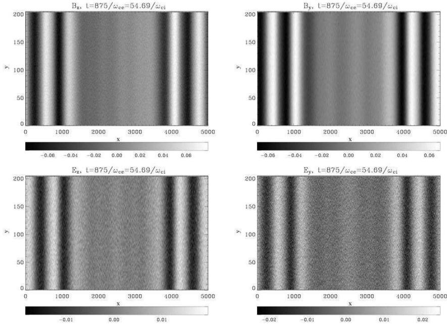
**Fig. 7.** As in Fig. 1 but for the case of homogeneous plasma density (no phase mixing). Note only non-zero (above noise level) components are plotted. There are no  $B_x$ ,  $E_x$  or density fluctuations present in this case.
