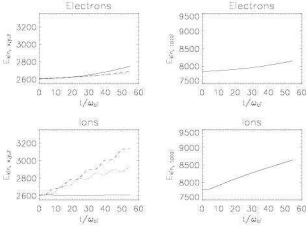
**Fig. 5.** Top row: kinetic energies (calculated by  $x$  (solid),  $y$  (dotted),  $z$  (dashed) velocity (squared) components) of electrons (left), and total kinetic energy for electrons (right) as a function of time. Bottom row: As above but for ions. The units on  $y$ -axis are arbitrary.
