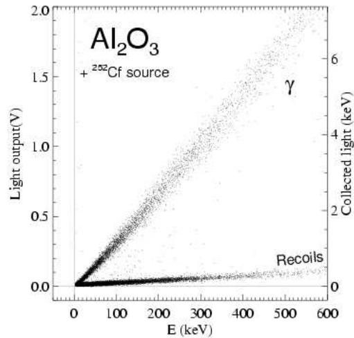
Figure 8. Discrimination between gammas and nuclear recoils in a 50 g sapphire bolometer at 20 mK by the ROSEBUD collaboration .
