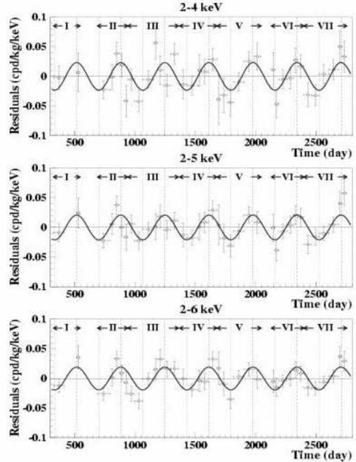
Figure 4. DAMA model independent residual count rates as a function of time for 7 years and three energy intervals (2-4), (2-5) and (2-6) keV-ee.
