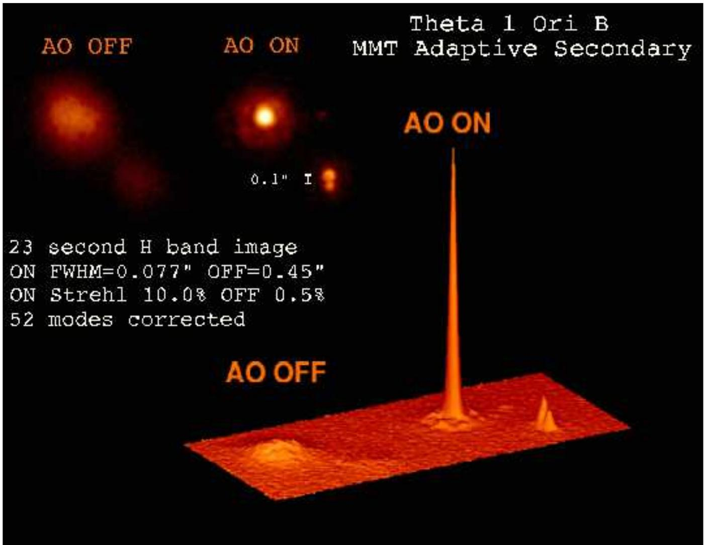
FIG. 1.— A typical example of how the the Adaptive Optics (AO) system can make very sharp images. With AO "OFF"  $\theta^1$  Ori B appears to be just 2 stars. With AO turned "ON" it is clearly a tight group of 4 visual stars. Note how with AO correction the peak intensity increases by 20 times and the resolution becomes ten times better.
