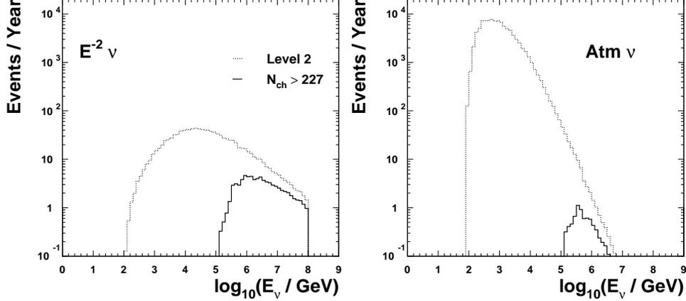
Fig. 9. **Energy spectra of selected neutrinos** for a  $E^{-2}$  source (*left*) and atmospheric neutrinos (*right*). The selection is given by level 2 cuts (dotted lines) and application of the optimized cut  $N_{\text{ch}} > 227$  (full lines). The cutoff in the signal spectrum at  $10^8$  GeV is due to the limited energy range of simulation.
