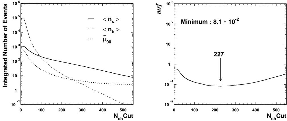
Fig. 8. **Cut optimization.** *Left:* Integrated distribution of detected channel multiplicity per event. *Right:* Model rejection factor with respect to a model source flux of  $E_\nu^2 \times dN_\nu/dE_\nu = 10^{-7} \text{ cm}^{-2} \text{ s}^{-1} \text{ sr}^{-1} \text{ GeV}$  as a function of the applied  $N_{\text{ch}} \text{ cut}$ .
