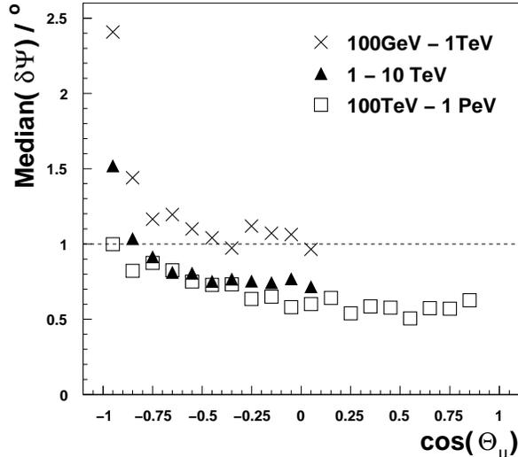
Fig. 6. **Pointing resolution for neutrino-induced muon events.** Shown is the median space angle error of the likelihood reconstruction as a function of the zenith angle of the incident track. The median was calculated for an energy spectrum  $\propto E^{-2}$  and after applying level 2 cuts.
