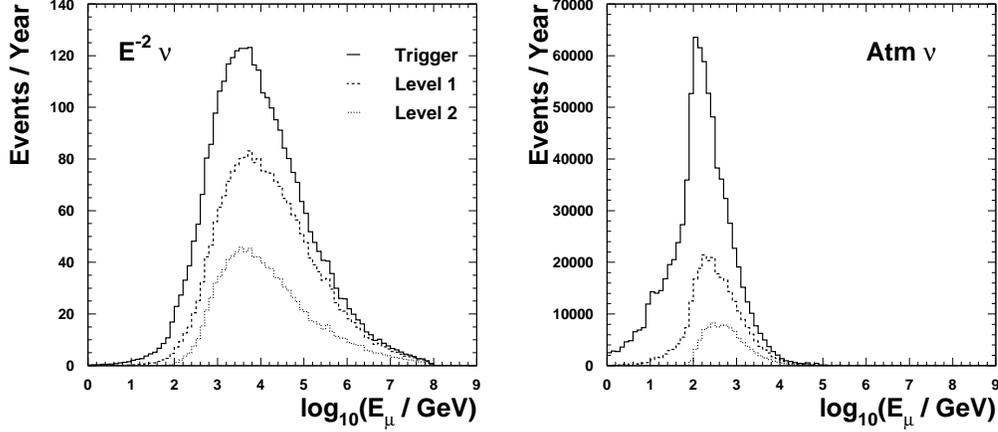
Fig. 3. Energy spectra of neutrino induced muons at different cut-levels: Signal from a  $E^{-2}$ -source (*left*), atmospheric neutrino background (*right*). The individual histograms in each plot correspond to: Trigger level (full lines), samples after applying level 1 cuts (dashed lines) and level 2 cuts (dotted lines). The energy spectra show the energy at the point of closest approach to the detector center.
