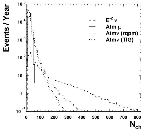
Fig. 4. Channel multiplicity for different event classes at level 2: For signal from  $E^{-2}$  source (dashed), atmospheric neutrinos including the two alternative charm contributions TIG (sparse dots) and rqpm (dense dots) and CR muon events (full lines).
