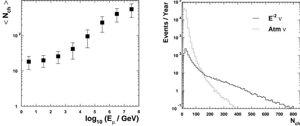
Fig. 7. **Channel multiplicity.** *Left:* Correlation between muon energy at closest approach to the detector center and detected channel multiplicity. Data points show to the mean number of OMs with a signal, averaged over one decade in energy. Error bars indicate the spread of the corresponding distribution. *Right:* Distribution of detected channel multiplicity for  $E^{-2}$  signal and atmospheric background.
