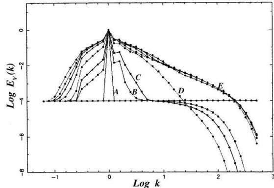
**Figure 1.** Turbulent kinetic energy per unit mass (in scaled units) as a function of wavenumber for various time in units of the eddy turnover time at  $k = 1$ . A: initial injection spectrum; B:  $t = 1$ ; C:  $t = 2$ ; D:  $t = 5$ ; E: curves for  $t = 10, 15, 20$  &  $30$ .
