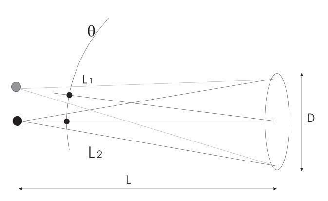
Fig. 1.— The observation of a light source at a distance L from the center of the telescope aperture. The distances between the source and two extremity positions on the aperture are denoted by  $L_1$  and  $L_2$ . A variation in  $L_1$  and  $L_2$  will result in an apparent displacement  $\Delta \theta$ in the location of the source .
