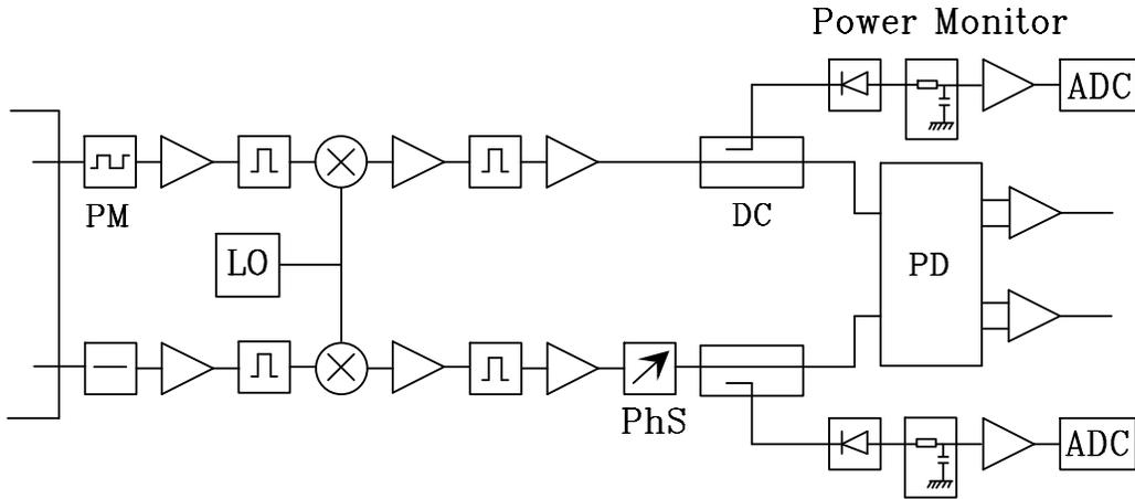
**Figure 3.** RF segment of the polarimeter: signal is phase modulated (PM), amplified, RF filtered and down-converted using a common local oscillator (LO). IF segment of the polarimeter: signal is amplified and filtered again. A phase shifter (PhS) is added in order to change the phase difference. A fraction of the signal is extracted by two directional couplers (DC) and used as Power Monitor.
