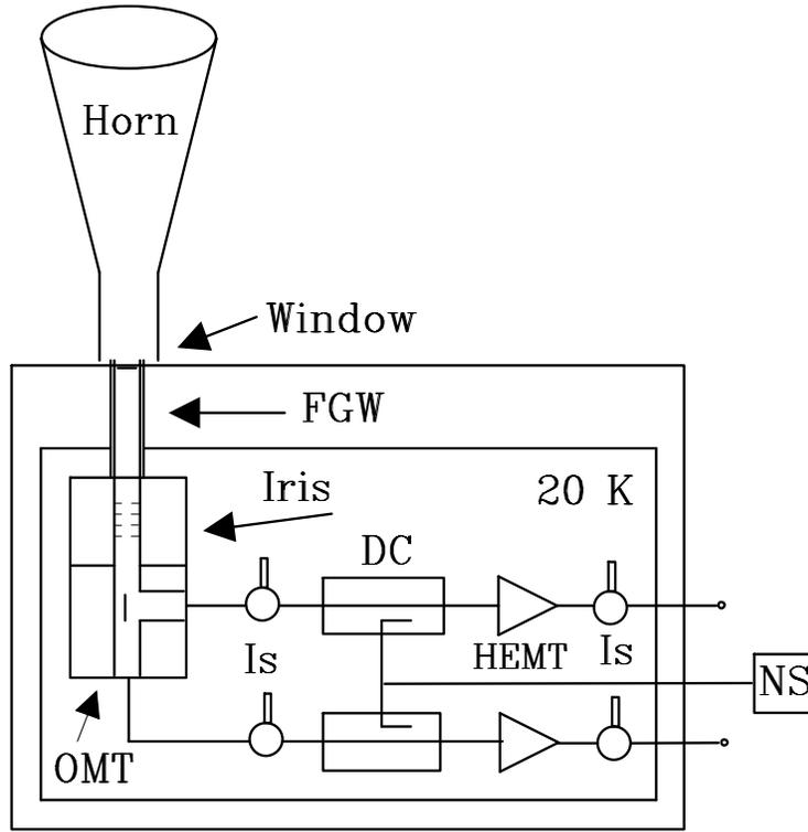
**Figure 2.** Front-end section of the polarimeter: Horn, Polyethylene Window, Fiber-glass Waveguide (FGW), Iris Polarizer, Ortho-mode transducer (OMT), cryogenic isolators (Is), directional couplers (DC) injecting the signal coming from the noise source (NS), and low noise HEMT amplifiers. The cryogenic components are operated at  $T \sim 20$  K.
