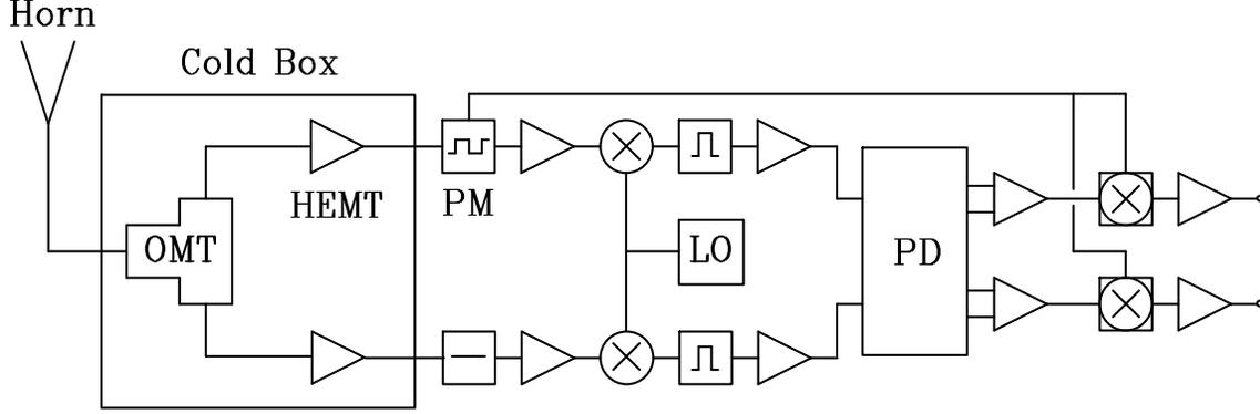
**Figure 1.** A schematic of the Milano polarimeter. The main blocks are shown: the cryogenic front-end, the modulation/demodulation loop, the RF-to-IF down-conversion, the Phase Discriminator.
