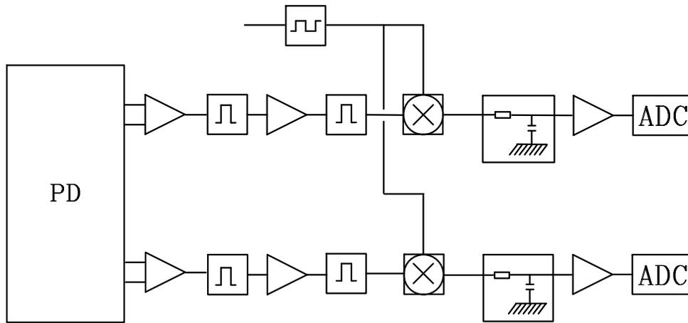
**Figure 5.** Post-detection segment of the polarimeter. The signal is filtered at the modulation frequency and amplified before the synchronous detection and the integration.
