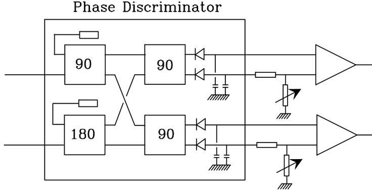
**Figure 4.** The phase discriminator: scheme of operation. The four hybrids are shown. The IF signal is detected by four crystal diodes. The amplification of the four signals is equalized by using a resistive partition.
