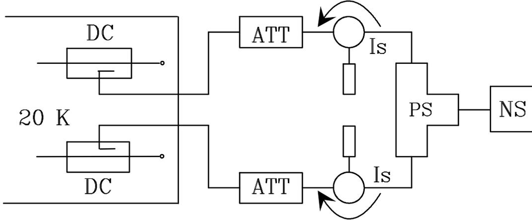
**Figure 6.** The internal calibration source. The signal from the noise source (NS) is divided by a power splitter (PS). In each chain we have an isolator (Is), a 30 dB attenuator (Att), and a directional coupler (DC) used to inject the signal into the amplification chains.
