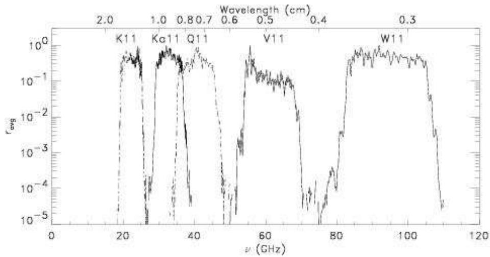
FIG. 8.— Combined responses,  $r_{avg}(v)$ , of representative radiometers in each of MAP's five frequency bands. Note that the frequency ranges of the Ka and Q band radiometers overlap slightly.
