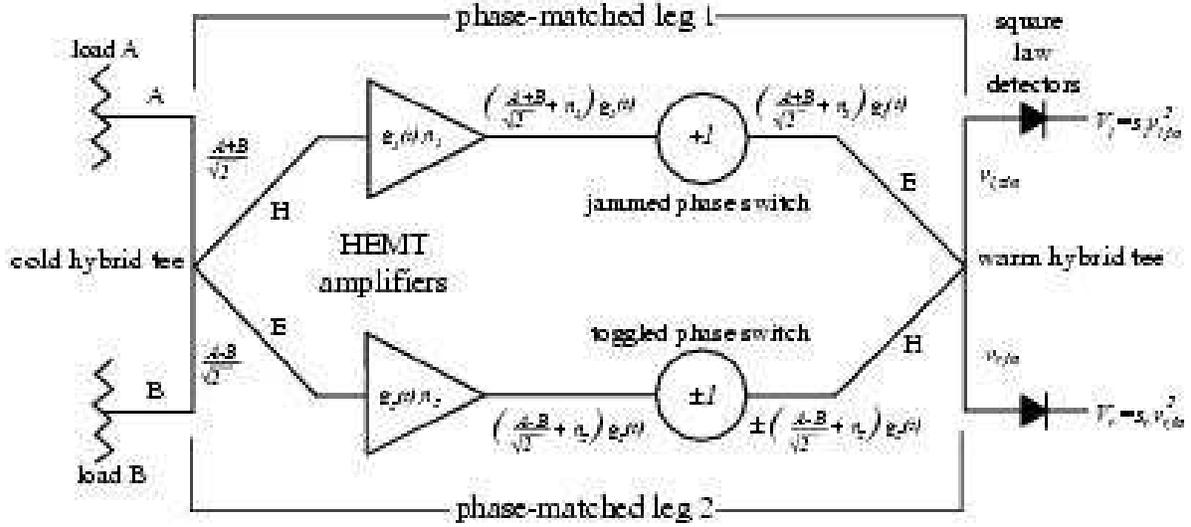
FIG. 3.— Simplified radiometer diagram used in the description of radiometer operation. The amplifiers' voltage gain and additive noise voltages are given by  $g_{1,2}(t)$  and  $n_{1,2}$ . The arms of the hybrid tees are labeled E and H. Expressions for signal levels are for voltages.
