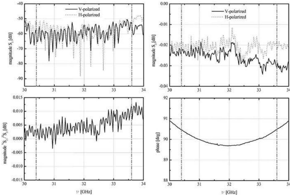
**Figure 7.** The characteristic of the polarizer. **Up left panel** shows the reflection coefficient at the input port of the polarizer. **Up right panel** reports the transmission coefficients ( $S_{21}$ ) of the two perpendicular polarizations. **Down left panel** shows the difference between the two  $S_{21}$  parameters. **Down right panel** is the phase difference between the two polarizations. Vertical dashed lines show the BaR-SPOrt bandwidth.
