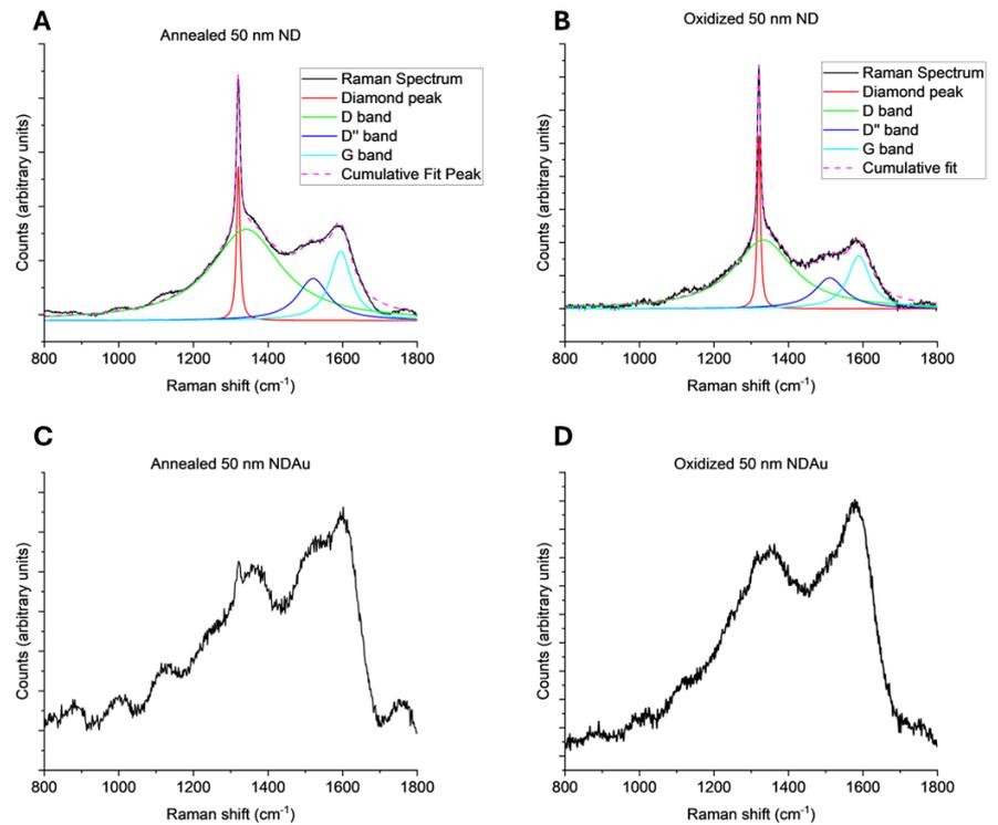
**Figure 3.2:** Raman spectra of 50 nm (A) Ann ND, (B) Ox ND, (C) Ann NDAu and (D) Ox NDAu. In unmodified nanodiamond spectra (A and B), 4 curves were deconvoluted from the spectra into the D peak (red), the D band (green), D'' band (dark blue) and G band (light blue).
