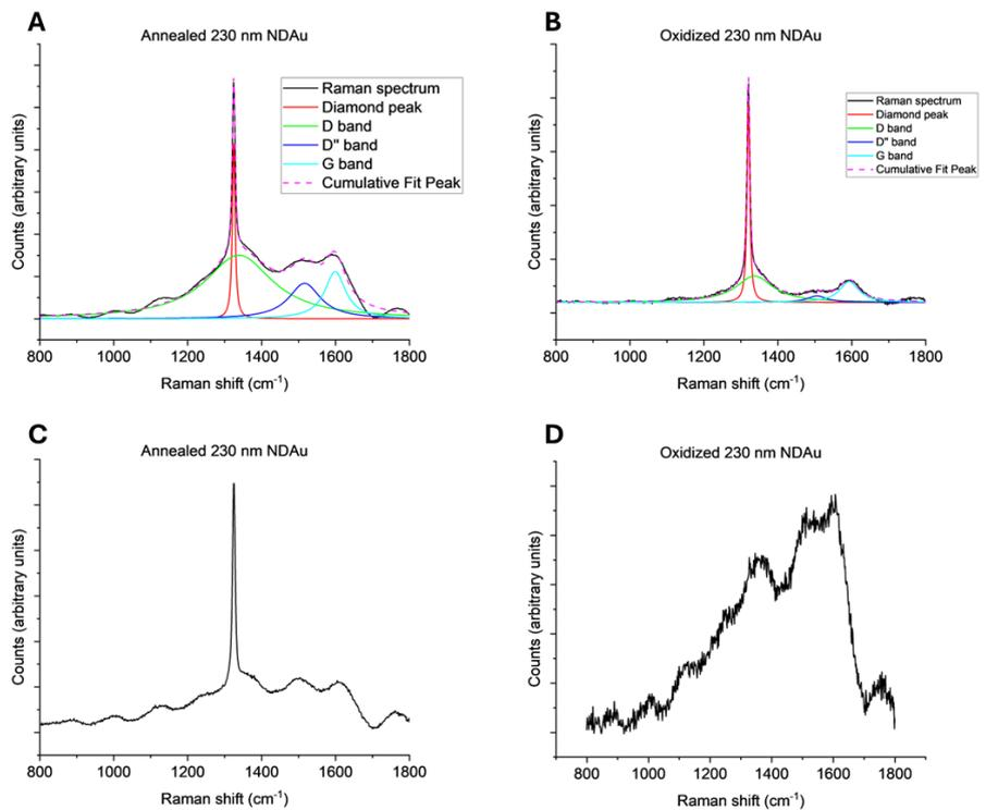
**Figure 3.3:** Raman spectra of 230 nm (A) Ann ND, (B) Ox ND, (C) Ann NDAu and (D) Ox NDAu. In unmodified nanodiamond spectra (A and B), 4 curves were deconvoluted
