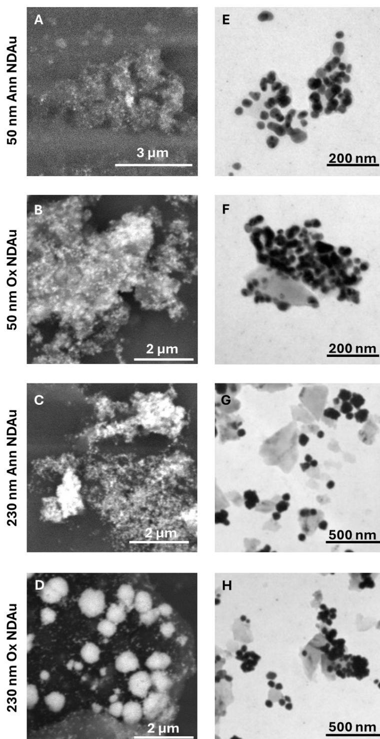
Figure 3.5. SEM (left) and TEM (right) images of NDAu annealed (Ann) and oxidized (Ox). 50 nm Ann NDAu (A,E); 50 nm Ox NDAu (B,F) 230 nm Ann NDAu (C,G); 230 nm Ox NDAu (D,H).
