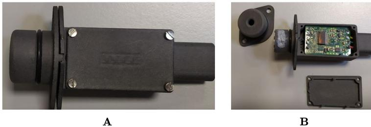
**Fig. 11** (A) Microgap sensor: assembled. (B) Opened, with electronics.
