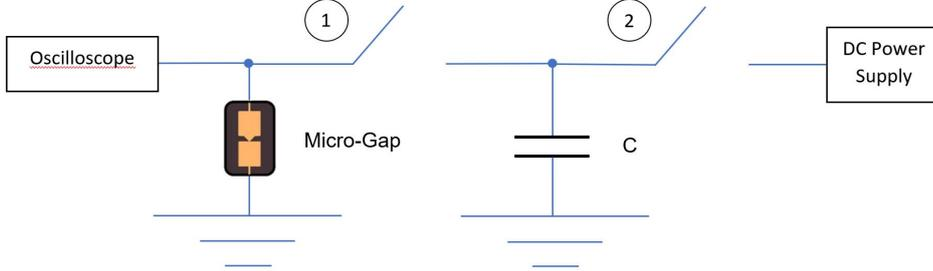
**Fig. 1** Functioning Blok Diagram. A capacitor is fully charged from power supply (switch 1 open, 2 closed), then it is connected to the Micro-Gap that allow electrical discharge (switch 1 closed and 2 open). The sensor allows to directly detect a possible decay of the dielectric strength of an insulating fluid.
