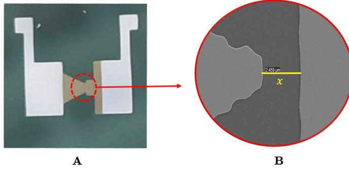
**Fig. 2** (A) Microgap made of a metal thin film, typically Cr 100 nm thick, deposited on an insulating layer ( $\text{SiO}_2$  or  $\text{Al}_2\text{O}_3$ ) with electric contacts (Al or Au, 150 nm thick). (B) Detail of the part of the device where the distance between electrodes is minimum. The spatial domain  $\Omega$  is set to represent the micro-gap extension.
