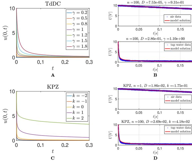
**Fig. 4** (A-C) TdDC and KPZ solutions at  $x = 0$ . Models parameters are set as  $D = 1$ ,  $n = 100$ ,  $U_0 = 10$ . (B-D) fitted solutions obtained through model calibration to experimental data.
