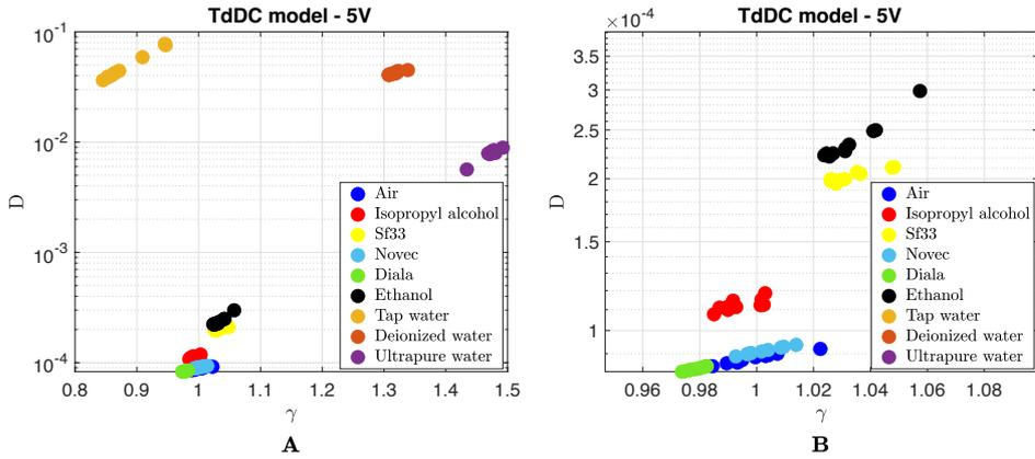
**Fig. 8** Optimal parameters obtained for conductive and insulating fluids, obtained from fitting the data on the voltage discharge observed when a 5 V electrical voltage to the micro-electrodes is applied.
