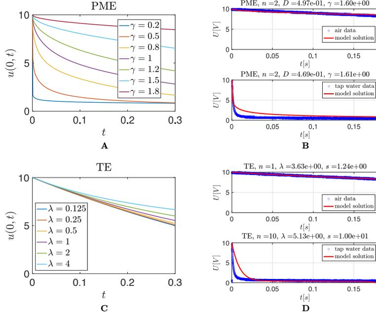
**Fig. 5** (A-C) PME and TE solutions at  $x = 0$ . Models parameters are set as:  $D = 1$ ,  $n = 100$ ,  $U_0 = 10$  (PME);  $s = 1$ ,  $n = 2$ ,  $U_0 = 10$  (TE). (B-D) Fitted solutions obtained through model calibration to experimental data.
