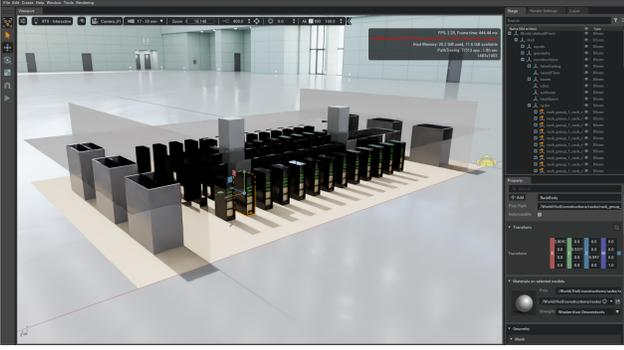
Fig. 4. Illustration of the layout of the considered DC with NVIDIA Omniverse. The data hall contains 4 rows of racks, with a total rack number equaling 60. 317 servers are installed in the racks. 6 ACU units are installed to provide cold air. Hot aisle containment is equipped to improve cooling efficiency.
