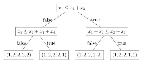
Figure 1: Decision tree for the LPT algorithm when m = 2 and n = 5 (with appropriate tie-breaking rules).
