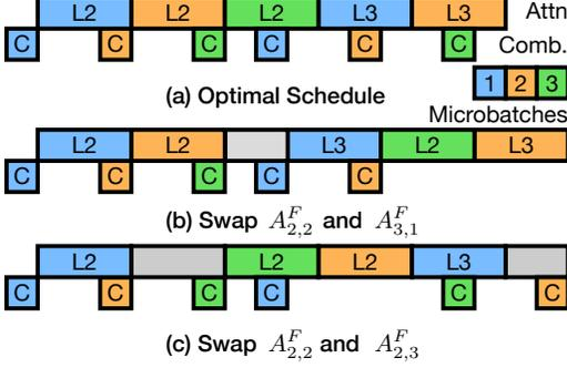
Figure 5: Demonstration of the optimal execution schedule of zebra parallelism, compared to swapping any of the two tasks. We show the forward attention computation and combine all-to-all of the second and third layers.
