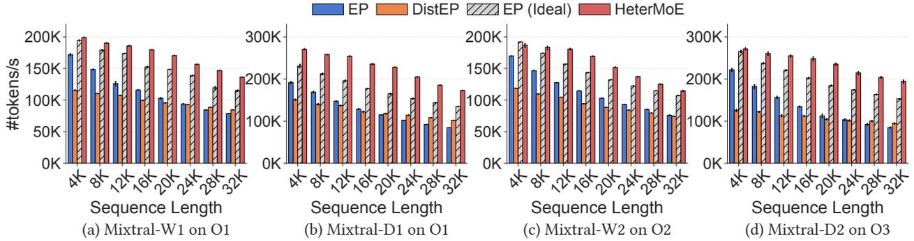
Figure 7: **[Overall Performance]**: Overall training throughput under different sequence lengths on the on-premise cluster of A40 and V100 GPUs, with different models and GPU setups. Error bars represent 95% confidence intervals.
