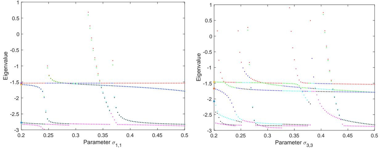
Figure 4: Results of changing parameters in an anisotropic choice of  $\Sigma$  for the hemispherical screen. We show changes in the smallest (in magnitude) target signatures as the parameters defining  $\Sigma$  given by (32) vary. Left panel: we set  $\sigma_{3,3} = 0.5$  and vary  $\sigma_{1,1}$ . Right panel: we set  $\sigma_{1,1} = 0.5$  and vary  $\sigma_{3,3}$ . Eigenvalues for different parameter values are shown as \*.
