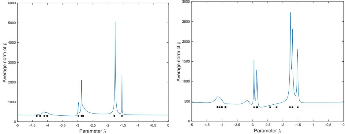
Figure 3: Predicted target signatures and computed  $\Sigma$ -Steklov eigenvalues for the hemisphere at  $\kappa = 1.9$ . Left: scalar  $\Sigma = 0.5iI$ . Right: anisotropic  $\Sigma$  with  $\sigma_1 = 0.5$  and  $\sigma_3 = 0.4$ . In each panel the curve shows the average of the norm of  $\mathbf{g}$  as the parameter  $\lambda$  varies, and the \* mark eigenvalues computed by FEM.
