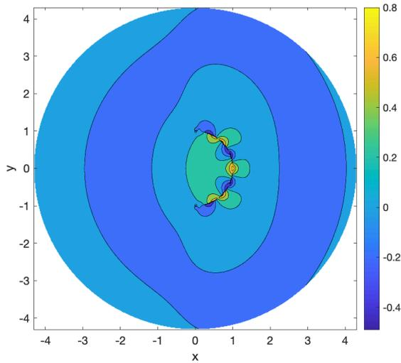
Figure 2: A contour map of the real part of the third component of the scattered electric field in the plane  $z = 0$ . Creeping waves along the screen are clearly visible. These waves have a shorter wavelength than the field in the bulk, so imposing an additional computational burden on the forward solver.
