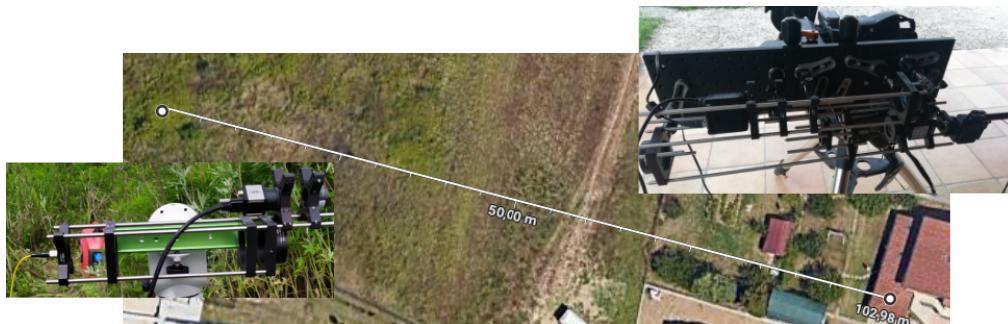
Fig. 3. The ground-to-ground channel in which the MAL was tested, with a photo of the transmitting (left) and of the receiving (right) system.
