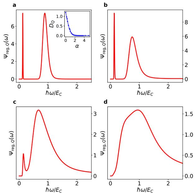
FIG. 4. QP model: regular part of the charge response function (in units of  $e^2\hbar/E_C^2$ ) as function of  $\frac{\hbar\omega}{E_C}$  at  $\beta E_C = 100$  and  $E_J/E_C = 0.5$  for  $\alpha = 0.3$  (a),  $\alpha = 0.9$  (b),  $\alpha = 2$  (c),  $\alpha = 4.2$  (d); in the inset of (a): charge Drude weight (in units of  $e^2/E_C$ ) as a function of  $\alpha$  at  $\beta E_C = 100$ .
