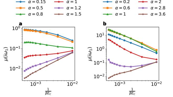
FIG. 7. Mobility along the imaginary axis: plot of the dimensionless mobility  $\mu(z)$  at the first Matsubara frequency  $z = i\omega_1 = i\frac{2\pi}{\beta\hbar}$ , for the CL model (a) and the QP model (b) for  $E_J/E_C = 0.5$ . In (a), the curves tend to 1 for  $\alpha \rightarrow 0$  as  $\omega_1$  approaches 0, while they decay to 0 for  $\alpha > \alpha_c$ . In (b), the mobility does not converge to 1 for  $\alpha \rightarrow 0$ .
