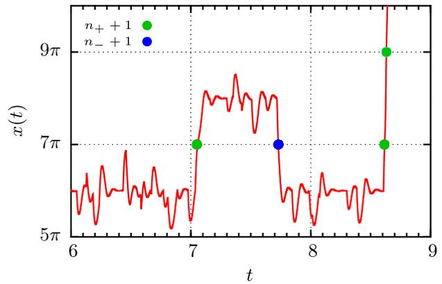
FIG. 7. A single exemplary trajectory of the system for the mass  $m = 0.017$ , the barrier height  $\varepsilon = 100$ , the mean spiking rate  $\lambda = 20$ , the average amplitude  $\zeta = 1/20$ , the variance  $\sigma^2 = 13$  and skewness  $\chi = 0.99$ . Colored dots correspond to the events of the periodic potential barrier crossing which translates to the increase in the counter  $n_{\pm}$ .
