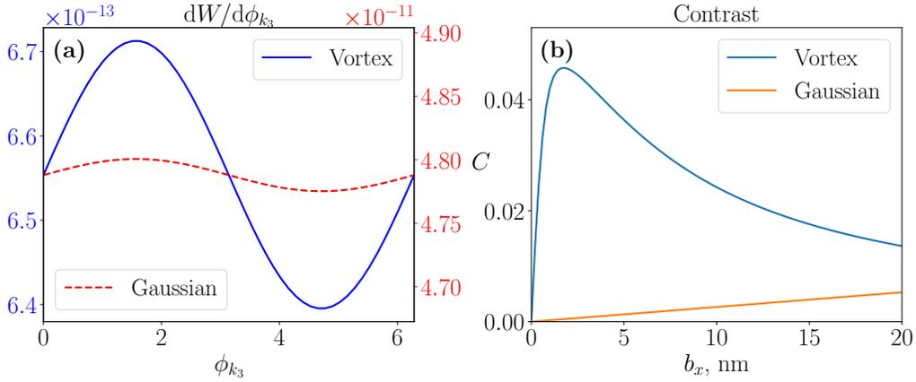
FIG. 12. (a): The distribution of the differential scattering probability with respect to the azimuthal angle  $\phi_{k_3}$  of the scattered electron. the impact parameters are set to  $b_x = 10$ nm and  $b_y = 0$ nm. Vortex particle scattering is represented by the left vertical axis, while Gaussian wave packet scattering is represented by the right vertical axis. (b): Dependence of the contrast  $C$  on the impact parameter  $b_x$ .
