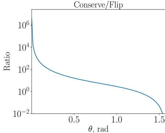
FIG. 13. The ratio of the differential scattering probabilities of spin-conserving to spin-flip as a function of  $\theta_{k_3}$ . In the figure, the azimuthal angle is fixed at  $\pi/2$ .
