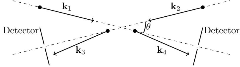
FIG. 7. Schematic of a non-collinear collision setup, where the crossing angle  $\theta$  is defined
