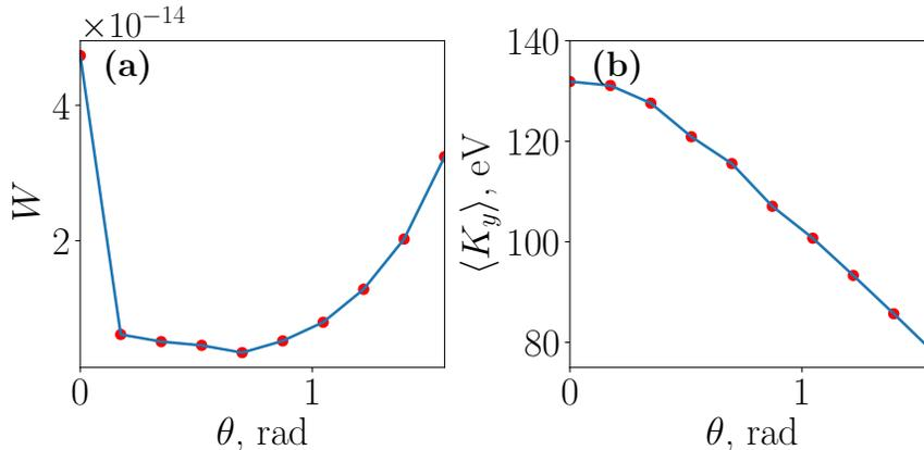
FIG. 9. The scattering probability (a) and the averaged total transverse momentum  $\langle K_y \rangle$  (b) are analyzed as a function of the crossing angle under non-collinear collisions. We set the impact parameters to  $b_x = 5\text{nm}$  and  $b_y = 0\text{nm}$ .
