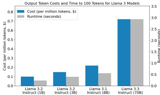
**Figure 10:** Comparison of output token costs (per million tokens) for the Llama 3 family on Amazon Bedrock and the time (in seconds) required to generate 100 tokens, measured on two NVIDIA H100 GPUs.
