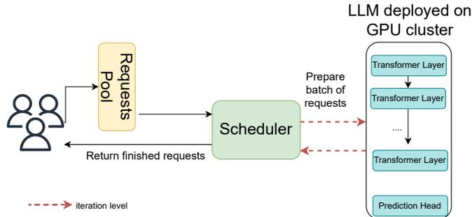
**Figure 6: Iteration-level scheduling.** The scheduler dynamically adjusts the batch and enables preemption decisions. After each token generation, it evaluates whether to continue with the current request or switch to another pending request. Finished outputs are returned to users as soon as they are ready.
