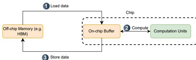
**Figure 5:** A neural network layer is executed on hardware devices by transferring data from memory (e.g., HBM) to on-chip buffers, then computing with the on-chip processing units, and eventually sending the output data back to memory.
