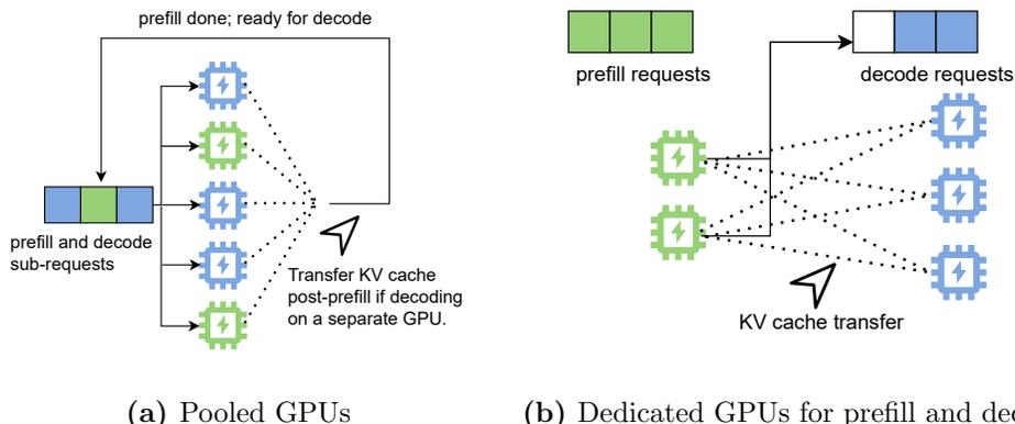
**Figure 7:** GPU organizations: comparing pooled GPUs with dedicated GPUs for prefill and decode phases.
