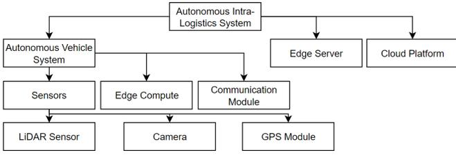
Fig. 6. **System component hierarchy.** Hierarchical representation of system components in the energy efficiency model, showcasing the relationships among AVs, edge servers, and cloud platforms.
