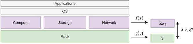
Fig. 4. **Measurement and validation process.** Measurements at different layers are compared and validated to ensure accuracy.
