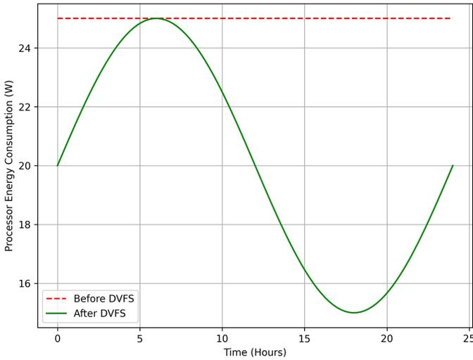
Fig. 8. **Impact of DVFS on processor energy consumption.** Shows a 20% reduction in energy consumption over time without affecting system responsiveness.
