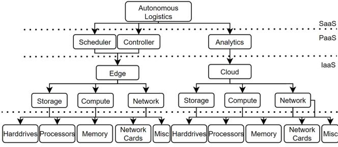
Fig. 2. **Software-Hardware Stack.** Mapping of software processes to underlying hardware resources in the edge-cloud continuum.
