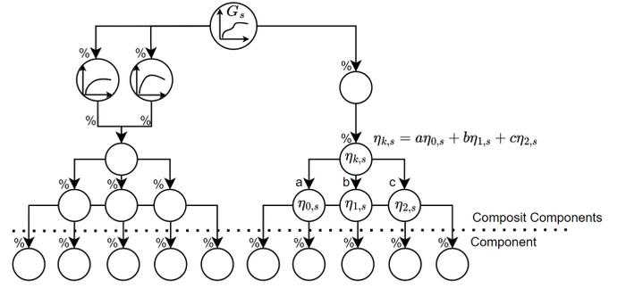
Fig. 3. **Energy efficiency graph.** Showing components and their interrelations within the system, resulting in the composite energy efficiency curves for the whole edge-cloud continuum example sketched in Figure 3.
