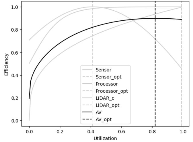
Fig. 7. **Synthetic component efficiency curves.** The curve illustrates energy efficiency and the peak utilization at 81% of an AV, when constructed as composite component based of three measurable components.
