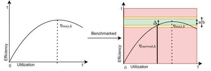
Fig. 5. **Efficiency curve for benchmarking.** Current utilization is located on the efficiency curve and related to the theoretical optimal efficiency, used for benchmarking the component.
