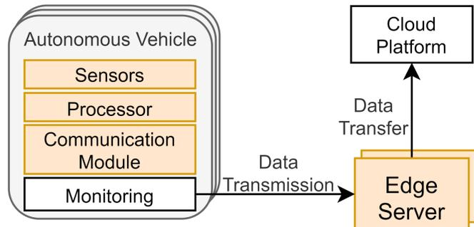
Fig. 1. **Energy consumption data flow.** The energy is measured on the autonomous vehicles and sent to edge computing via the network. The edge computing and network energy is derived from utilization and measurement. All data is sent to the cloud for further processing and analysis.
