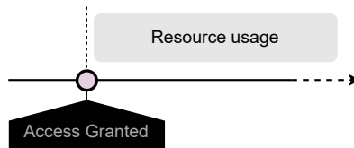
Fig. 2 The enforcement process of an access control system. There is no further control after access has been granted and the resource is used.
