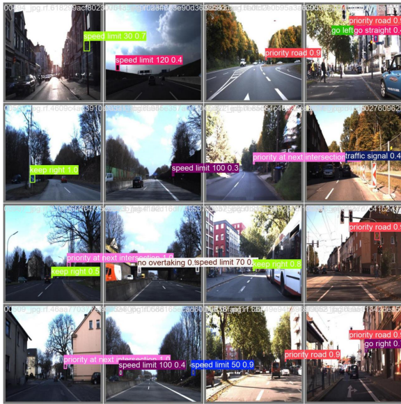
Figure 6. YOLOv8-Based Traffic Sign Detection results on real-world scenes. The model detects multiple signs (bounding boxes) in diverse conditions, demonstrating high recall and precision.
