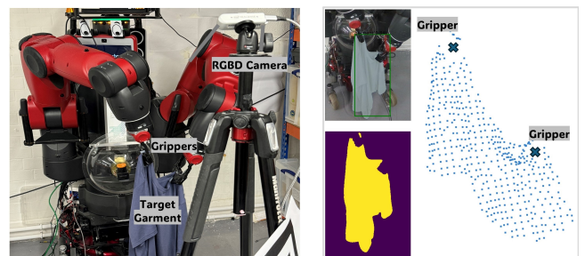
Fig. 7. Real-world setup for cloth garment dynamics prediction task: A Baxter robot is used for garment manipulation. The results of Grounded SAM and the projected point cloud are also demonstrated here.
