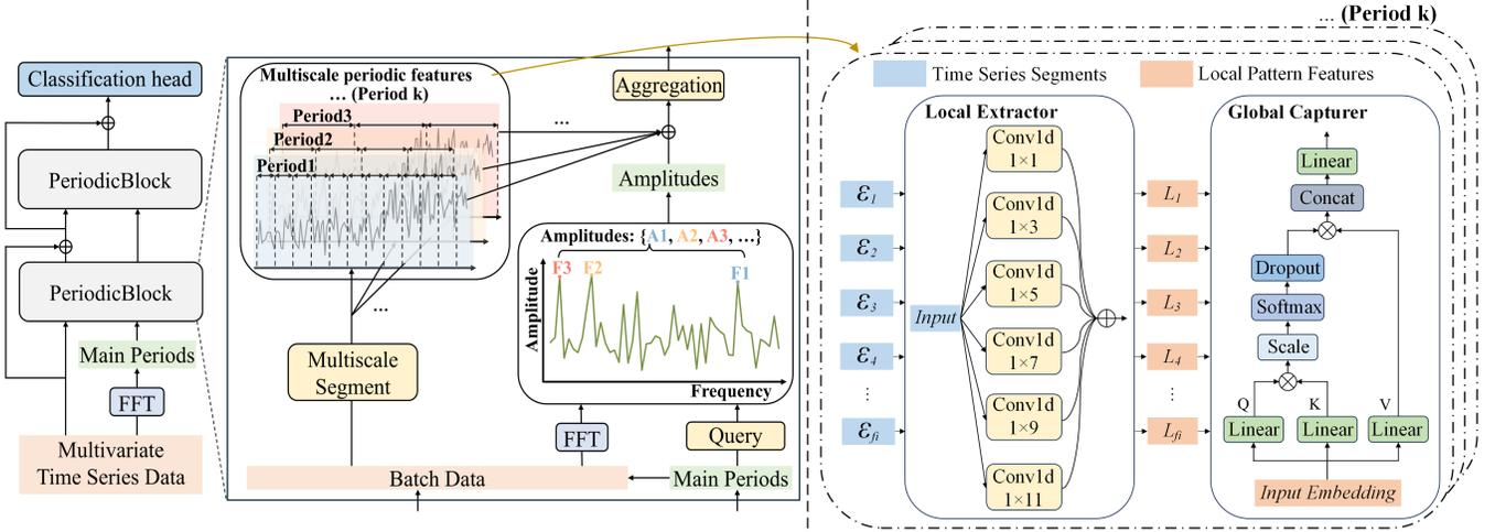
Figure 3: Overview of the Multiscale Periodic Time Series Network (MPTSNet). The model processes multivariate time series data through FFT to identify the main periods. The data is then segmented into multiscale periodic components, where Local Extractor and Global Capturer in PeriodicBlock extract features sequentially at different scales. The features are aggregated by corresponding amplitudes and passed through the Classification head for final prediction.
