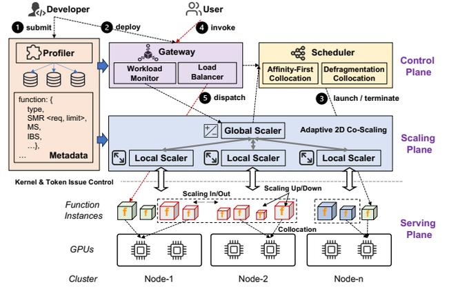
**Figure 3.** The system architecture of Dilu.
