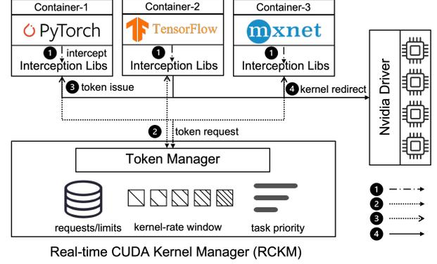
**Figure 6.** The vertical scaling workflow in Dilu.
