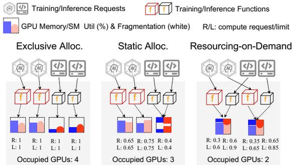
Figure 1. GPU provisioning of serverless DL systems.
