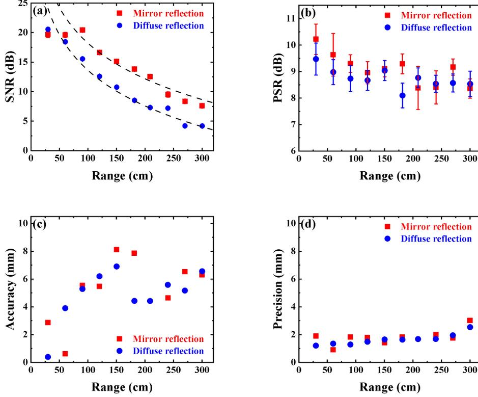
**Fig. 4.** (a) SNR, (b) PSR, (c) accuracy, and (d) precision of the mid-infrared chaos lidar versus the target range. Squares denote the mirror reflection and dots denote the diffuse reflection. The error bar stands for the standard deviation of the repeated measurements. The dash lines in (a) are least-squares fitting curves of the measured results using the reciprocal of quadratic function.
