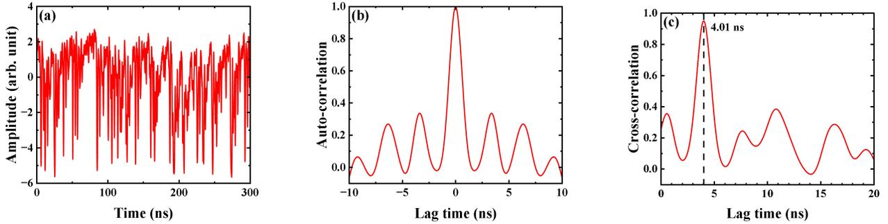
**Fig. 3.** (a) Temporal waveform, (b) autocorrelation, and (c) cross-correlation of the ICL chaos. The cross-correlation peak at 4.01 ns in (c) translates into a target distance of 60.1 cm.
