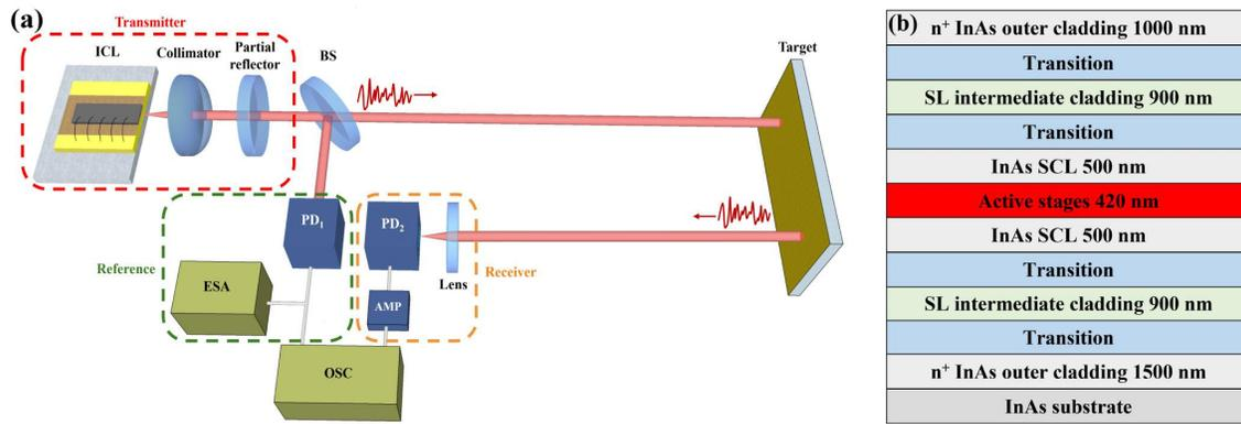
**Fig. 1.** (a) Experimental setup of the mid-infrared chaos lidar. BS: beamsplitter; PD: photodetector; AMP: amplifier; ESA: electrical spectrum analyzer; OSC: oscilloscope. (b) Epitaxial layer structure of the InAs-based ICL.
