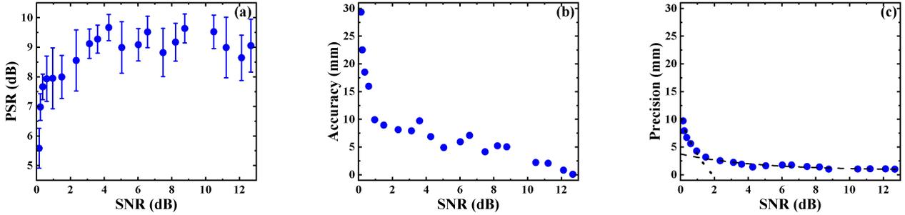
**Fig. 5.** Impact of the SNR on (a) the PSR, (b) the accuracy, and (c) the precision of the mid-infrared chaos lidar. The target distance is 150.3 cm, and the reflection is diffuse reflection. The dot line in (c) denotes the least-squares fitting using the reciprocal of the quadratic function, and the dash line denotes the fitting using the reciprocal function.
