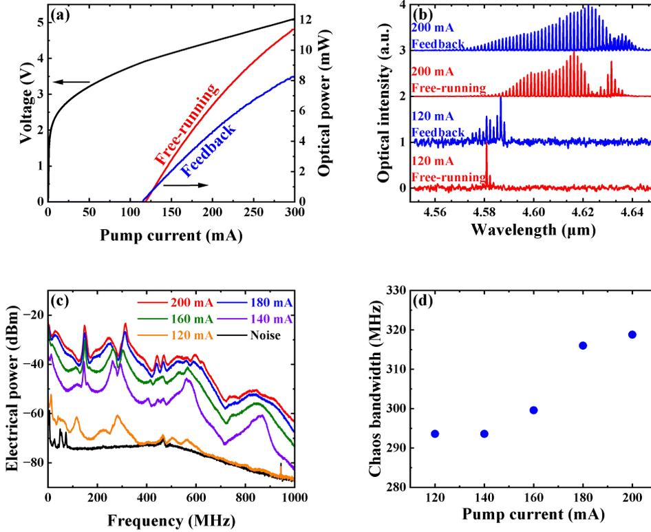
**Fig. 2.** (a) L-I-V curves and (b) optical spectra of the ICL with and without optical feedback. (c) Chaos spectra and (d) chaos bandwidth for various pump currents.
