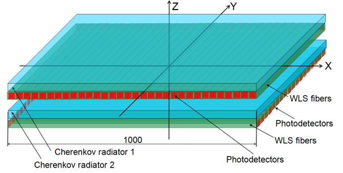
Fig. 3. Schematic design of a Cherenkov photon detector with WLS-fiber readout (not to scale).
