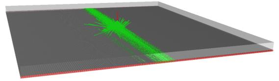
Fig. 5. Visualizations of muon interactions with one of the Cherenkov radiator ( $30 \times 1000 \times 1000 \text{ m}^3$ ) were simulated in GEANT4 for a configuration with a 2 mm square-shaped WLS fiber array and SiPMs ( $2 \times 2 \text{ mm}^2$ ) for the optical readout of the fibers. The muon impinges on the detector from the side of the radiator, producing light in the WLS fibers.
