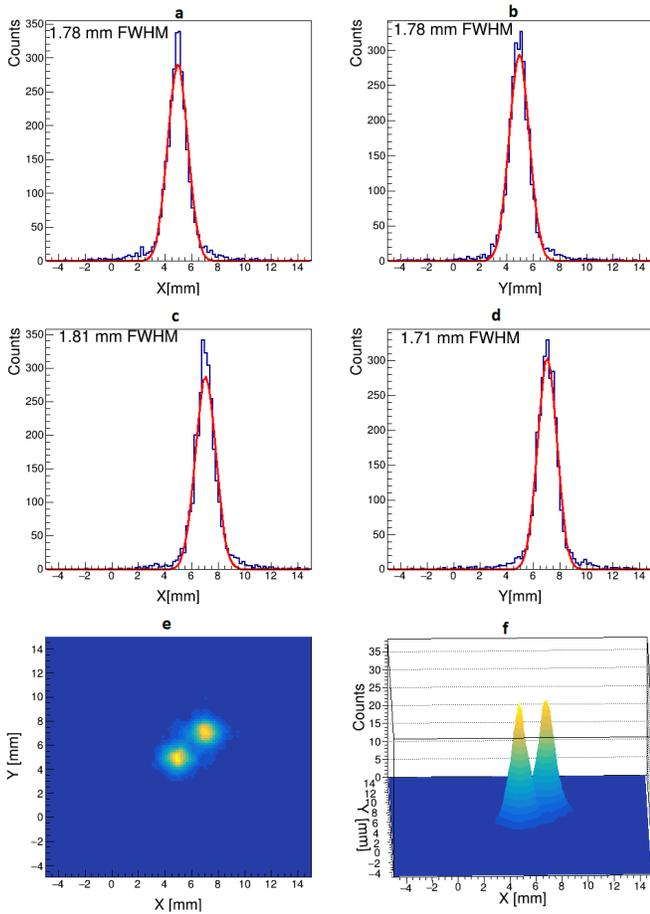
Fig. 8. Reconstructed muon interaction positions for two muon beam positions impinging on the central detector area, with profiles along the  $x$ -axis and  $y$ -axis (a-d), show position resolutions of 1.8 mm (FWHM). The sigma value of the fitted Gaussian waveform can be considered as the position resolution. Reconstructed muon interaction positions in 2D (e) and 3D (f) representations. Two muon beam coordinates are  $x_1 = 5$  mm,  $y_1 = 5$  mm and  $x_2 = 7$  mm,  $y_2 = 7$  mm.
