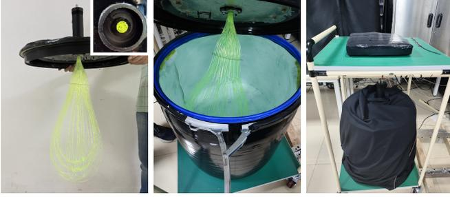
Fig. 2. (a) Fiber-PMT assembly mounted on the tank lid. The top right corner shows the milled fiber ends. (b) The tank, filled with filtered water; the inner surface was lined with Tyvek 1085D, and the fibers are submerged. (c) Configuration of the experimental setup. Dual trigger detectors are positioned above and below the WCD. The figures are taken from [22]
