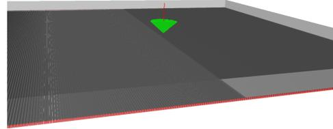
Fig. 6. Visualizations of muon interactions with one of Cherenkov radiators were simulated in GEANT4 for a configuration with a 2 mm square-shaped WLS fiber array and SiPMs ( $2 \times 2 \text{ mm}^2$ ) for the optical readout of the fibers. The muon impinges on the detector from the side of the WLS fibers, producing a cone of light in the direction of the black-painted surface of the radiator, thus not generating light in the WLS fibers.
