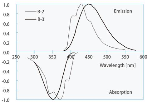
Fig. 4. Absorption and Emission Spectra for the WLS fiber used for the light collection of the Cherenkov light (Kurary WLS Fiber Data Sheet).
