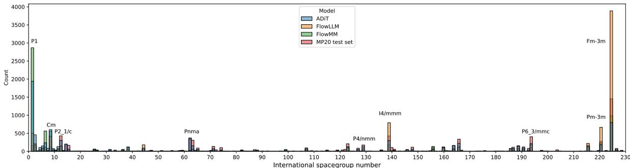
**Figure 5 Histogram of spacegroups for 10,000 generated crystals.** Diffusion-based ADiT and FlowMM tend to over sample crystals with P1 spacegroup compared to the MP20 training distribution. FlowLLM, an autoregressive language, tends to over sample crystals with Fm-3m, Pm-3m, and I4/mmm spacegroups.
