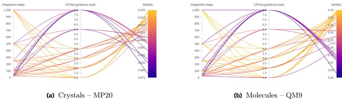
**Figure 7 Tuning inference hyperparameters for best performance.** Best generative modelling results for crystals and molecules are achieved with different classifier-free guidance scales  $\gamma$  and number of integration steps  $T$ .  $T = 500$  or 1000 with  $\gamma = 1.0$  or 2.0 tends to work well across both molecules and crystals.
