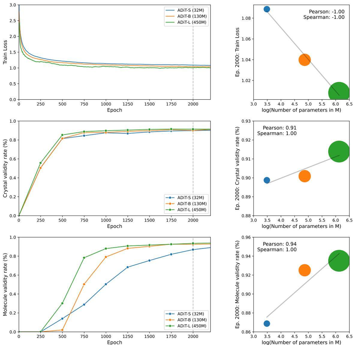
**Figure 3 Scaling up ADiT improves performance.** We show the effect of increasing the number of ADiT denoiser parameters on the training loss and generation validity rates. *Left:* training loss and validity rates vs. epochs. *Right:* Correlation plots for training loss and validity rates at epoch 2,000 vs. ADiT parameters (in Millions).
