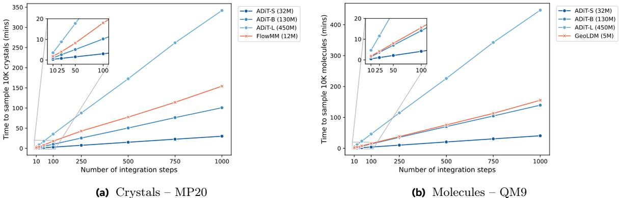
**Figure 2 ADiTs are significantly faster than equivariant diffusion models.** We plot the validity rate vs. number of integration steps for ADiTs and equivariant diffusion models for generating 10,000 samples on a single V100 GPU. ADiTs scale significantly better with the number of integration steps compared to equivariant diffusion.
