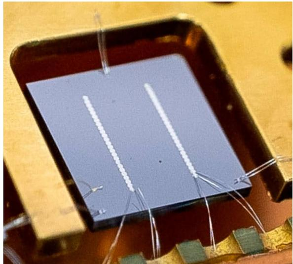
FIG. 1. The TESSERACT  $1 \text{ cm}^2$  detector used in this analysis [33]. The detector is supported by wirebonds attached at the top center and bottom corners of the detector. A gold wirebond (left side) is used to cool the detector. The two sensor channels (“left” and “right”) can be seen as the parallel lines, each biased and read out separately (see electrical wirebonds to readout PCB).
