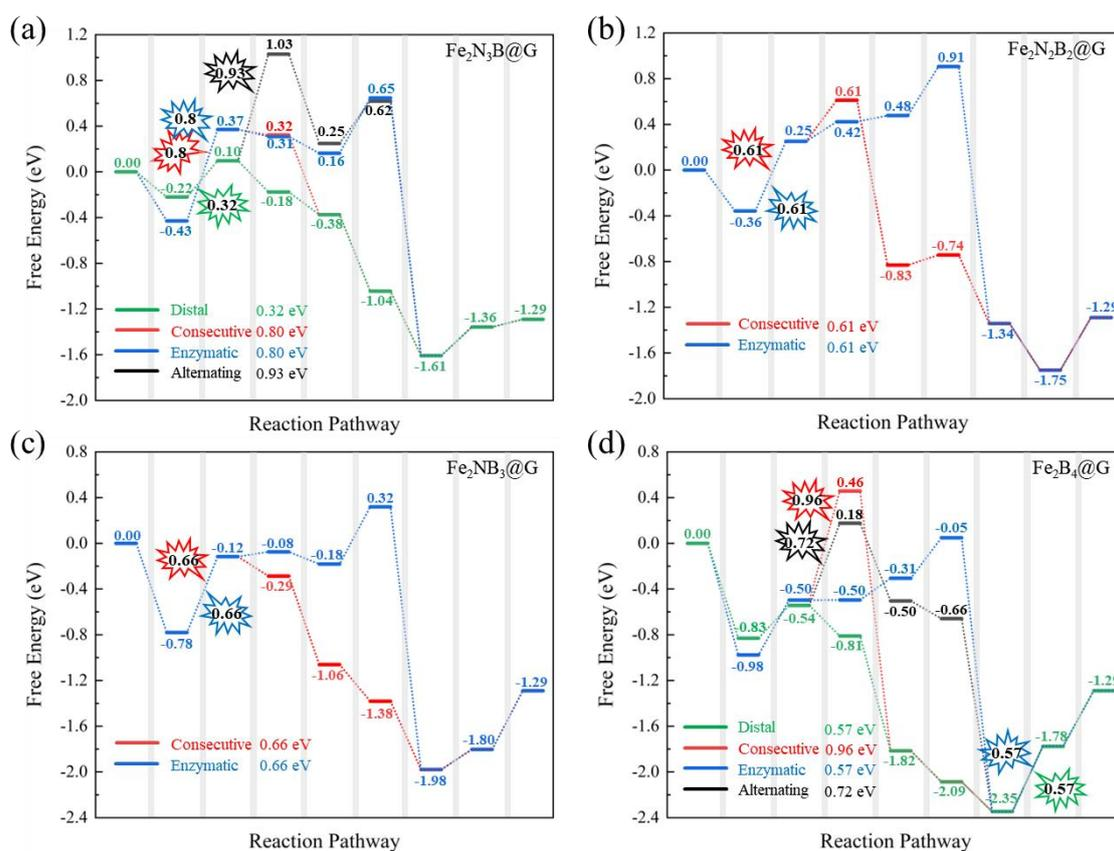
**Figure 2.** Free energy changes of the distal, alternating, consecutive and enzymatic pathways of NRR on catalysts of (a)  $\text{Fe}_2\text{N}_3\text{B}@G$ ; (b)  $\text{Fe}_2\text{N}_2\text{B}_2@G$ ; (c)  $\text{Fe}_2\text{NB}_3@G$ ; (d)  $\text{Fe}_2\text{B}_4@G$ .
