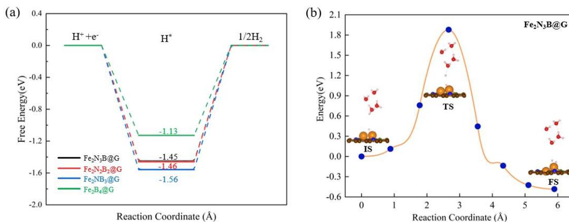
**Figure 6.** (a) Free energy curves of HER on  $\text{Fe}_2\text{N}_3\text{B}$ ,  $\text{Fe}_2\text{N}_2\text{B}_2$ ,  $\text{Fe}_2\text{NB}_3$ , and  $\text{Fe}_2\text{B}_4$  catalysts. (b) Minimum energy pathway for  $\text{H}_2$  generation on  $\text{Fe}_2\text{N}_3\text{B}@G$  catalyst.
