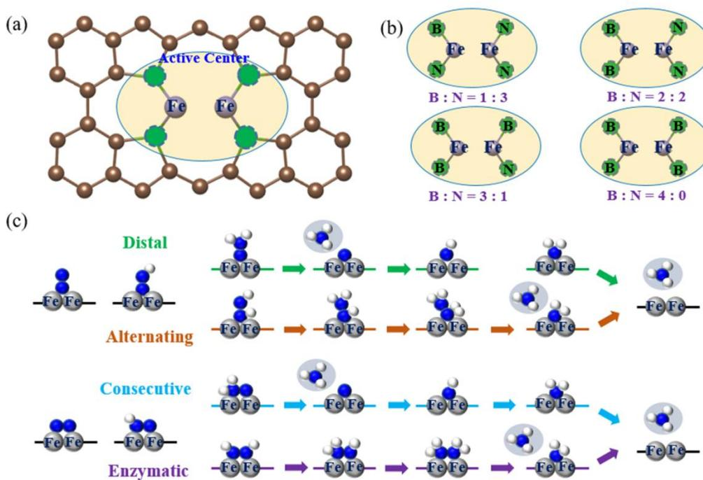
**Figure 1.** (a) Schematic diagrams of the crystal structures of the dual-Fe atomic catalyst anchored on boron-nitrogen doped graphene. (b) The doping structure with different ratios of B vs N. (c) Schematic diagrams of the four different pathways of NRR, including distal, alternating, consecutive and enzymatic pathways.
