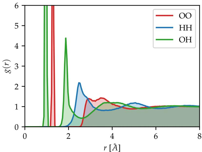
**Figure 3** Radial distribution function between oxygen atoms (OO), hydrogen atoms (HH) and oxygen-hydrogen pairs (OH) calculated using 512  $\text{H}_2\text{O}_2$  molecules in the liquid phase at 300 K and 1 atm.
