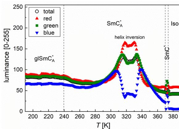
Figure S2. Average weighted luminance and separate contributions of the red, green, and blue components of the POM textures of 3F5HPhF6 obtained on cooling at 10 K/min in the transmission mode.
