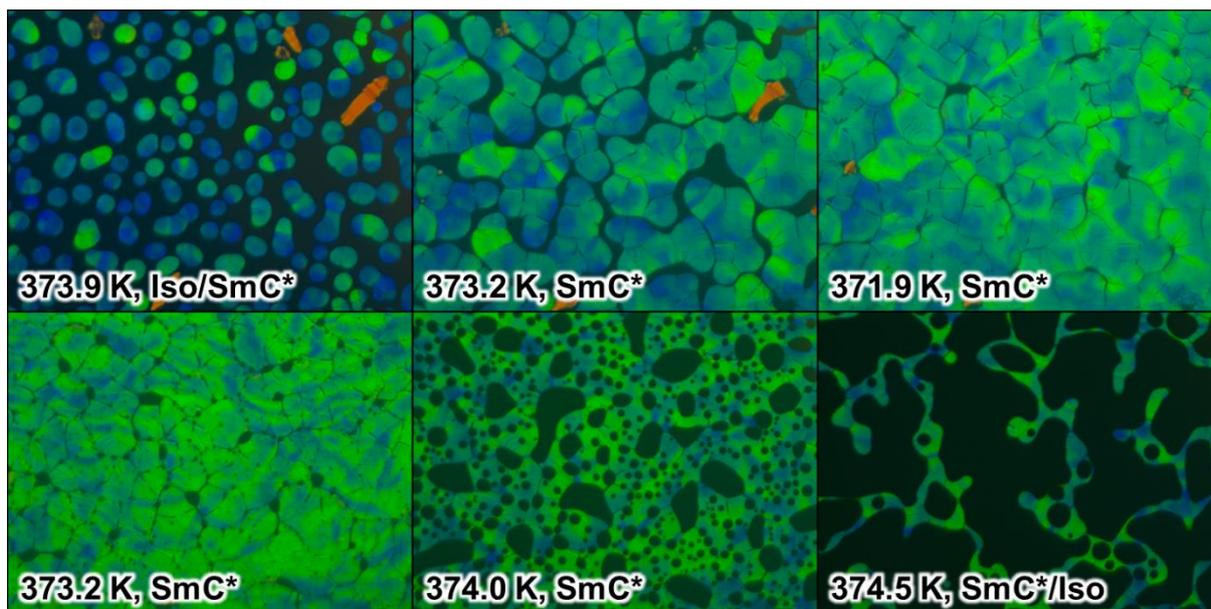
Figure S7. POM textures of 3F5HPhF6 registered on cooling (upper row) and heating (bottom row) at 1 K/min in the reflection mode. Each image shows an area of  $622 \times 466 \mu\text{m}^2$ .
