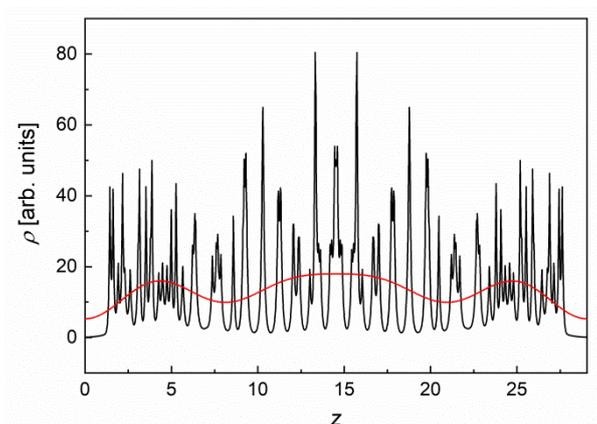
Figure 10. Centrosymmetric electron density distribution of 3F5HPhF6 based on the DFT calculations (B3LYP-D3(BJ), def2TZVPP) along the smectic layer normal. The red line is the fitting result of Equation (4).
