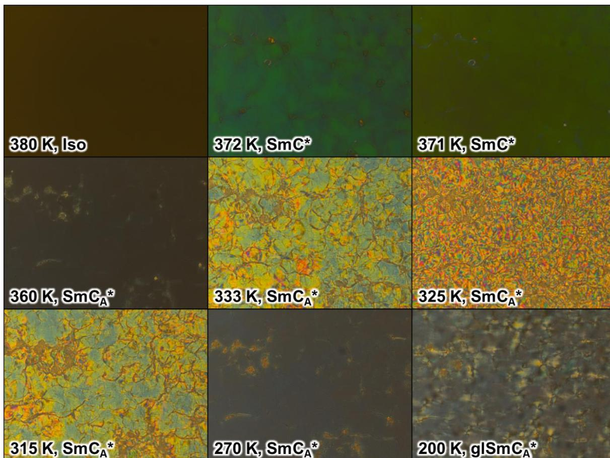
Figure S1. POM textures of 3F5HPhF6 registered on cooling at 10 K/min in the transmission mode. Each image shows an area of  $1243 \times 933 \mu\text{m}^2$ .
