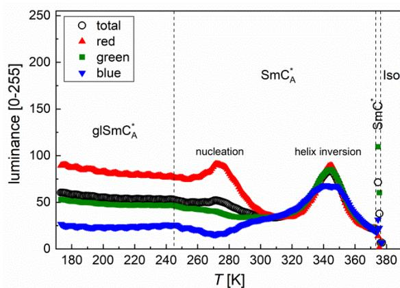
Figure S6. Average weighted luminance and separate contributions of the red, green, and blue components of the POM textures of 3F5HPhF6 obtained on heating at 10 K/min in the reflection mode.
