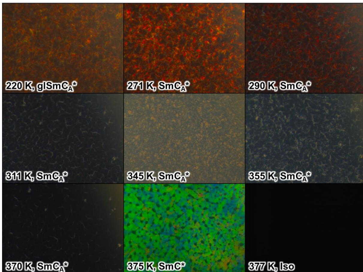
Figure S5. POM textures of 3F5HPhF6 registered on heating at 10 K/min in the reflection mode. Each image shows an area of  $622 \times 466 \mu\text{m}^2$ .
