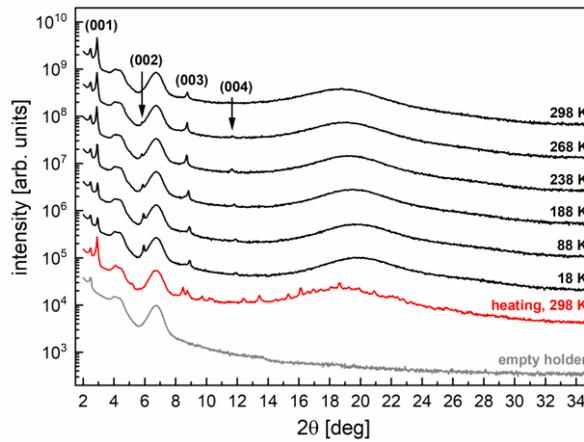
Figure 5. Selected XRD patterns of 3F5HPhF6 collected on cooling from 298 K to 18 K and after gradual heating to 298 K. The bottom pattern was collected at room temperature for an empty holder. The sharp peaks arising from the smectic layer order are indicated.
