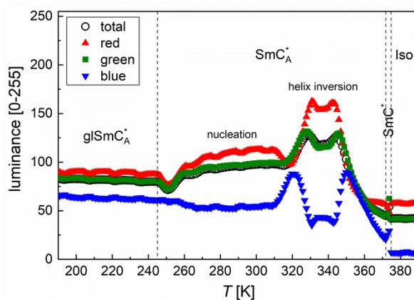
Figure S4. Average weighted luminance and separate contributions of the red, green, and blue components of the POM textures of 3F5HPhF6 obtained on heating at 10 K/min in the transmission mode.
