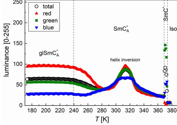
Figure 4. Average weighted luminance and separate contributions of the red, green, and blue components of the POM textures of 3F5HPHF6 obtained on cooling at 10 K/min in the reflection mode.
