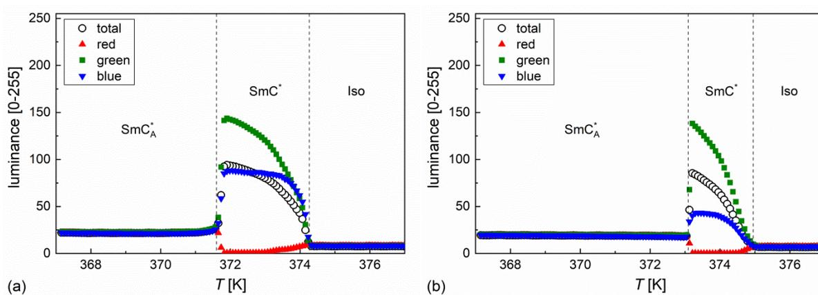
Figure S8. Average weighted luminance and separate contributions of the red, green, and blue components of the POM textures of 3F5HPhF6 obtained on cooling (a) and heating (b) at 1 K/min in the reflection mode.
