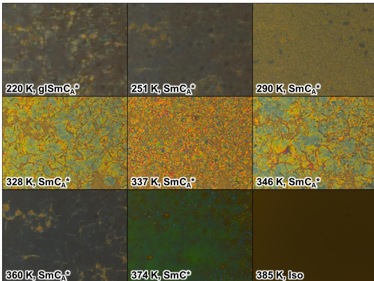
Figure S3. POM textures of 3F5HPhF6 registered on heating at 10 K/min in the transmission mode. Each image shows an area of  $1243 \times 933 \mu\text{m}^2$ .
