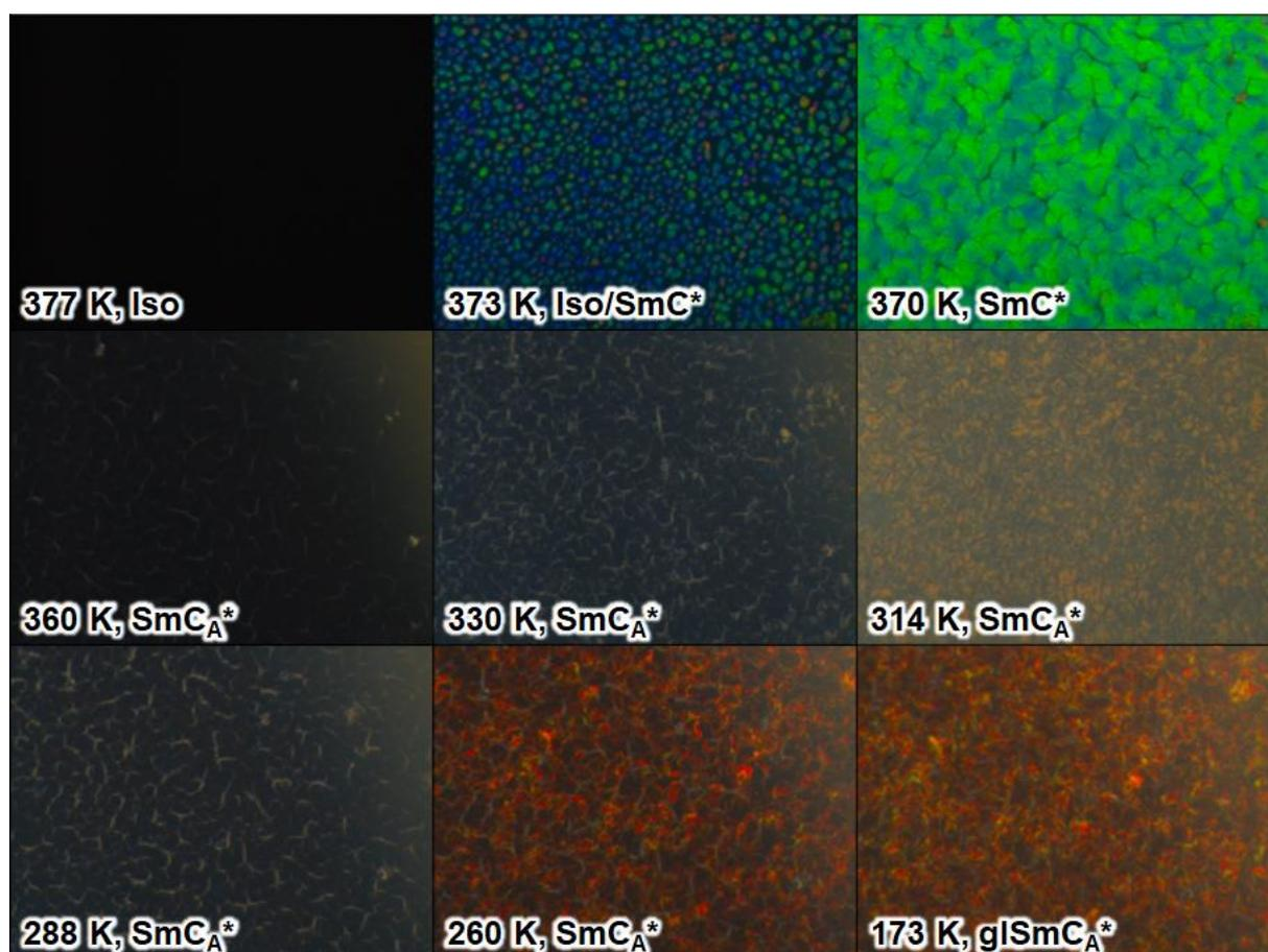
Figure 3. POM textures of 3F5HPhF6 registered on cooling at 10 K/min in the reflection mode. Each image shows an area of  $622 \times 466 \mu\text{m}^2$ .
