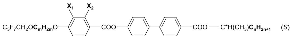
Figure 1. The general molecular formula of 3FmX<sub>1</sub>PhX<sub>2</sub>n. In this work, m = 5, X<sub>1</sub> = H, X<sub>2</sub> = F, n = 6.
