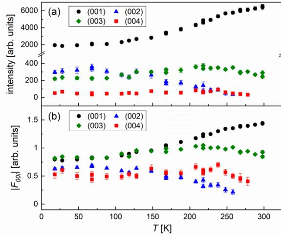
Figure 7. Integrated intensities of the (00*l*) peaks from the smectic layers of supercooled and vitrified 3F5HPhF6 (a) and the absolute values of the structure factors, calculated from these intensities after correction by the Lorentz-polarization factors (b).
