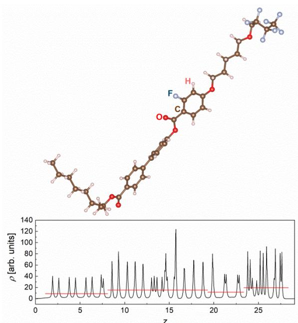
Figure 9. The model of the 3F5HPhF6 molecule optimized by the DFT method (B3LYP-D3(BJ) functional, def2TZVPP basis set) and the corresponding electron density profile projected on the smectic layer normal, oriented in the horizontal direction. The red lines indicate the average electron density for various molecular parts.
