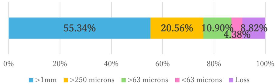
Figure 5 Sieved size fractions as percentage of original particle by mass.
