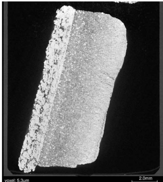
Figure 1 Tomographic cross section of the iron ore particle studied in this work.
