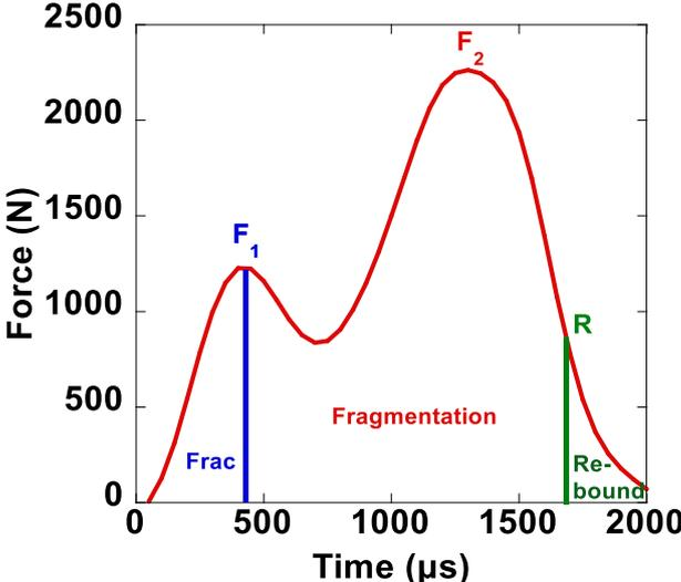
Figure 4 Impactor inertial force during breakage showing the two stages of breakage: fracturing and fragmentation.
