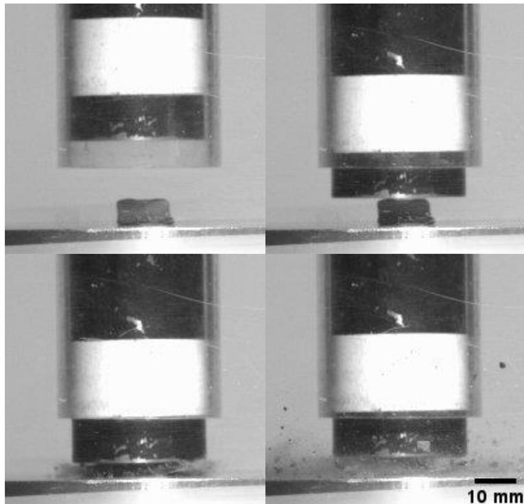
Figure 3 Single frames from highspeed video of breakage of iron ore particle. Top left: Before breakage. Top right: Frame of contact between impactor and particle. Bottom left: Frame of minimum height of impactor above base, where velocity reverses to rebound. Bottom right: Height of impactor rebound and expulsion of particle fragments.
