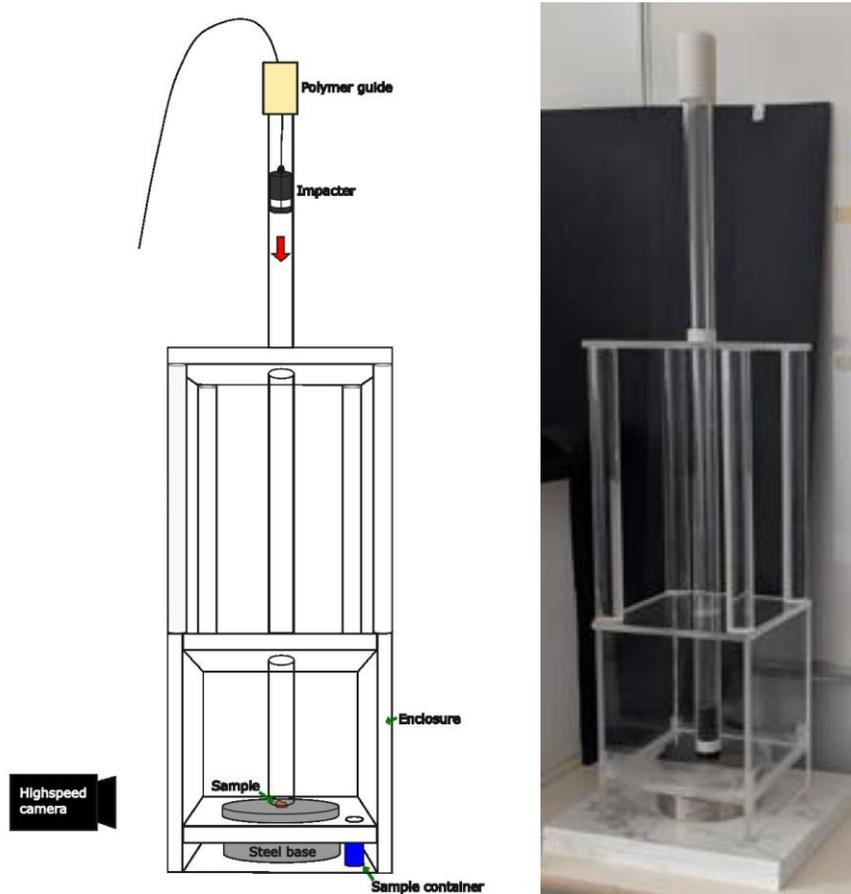
Figure 2 Left: Schematic drawing of custom drop weight test. Right: Photo of lab setup of custom drop weight test.
