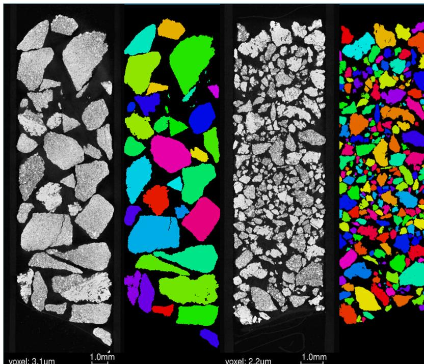
Figure 6 Tomographic slices and labelled fragments. Left: Fragments >1mm. Right: Fragments >250 microns.
