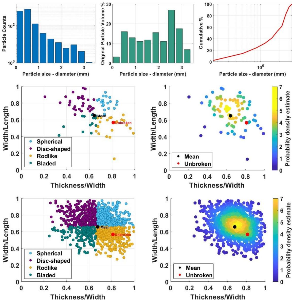
Figure 7 Fragment size and shape analysis. Top (left to right): Particle size by particle counts, particle size by volume, probability density function of particle size. Middle: Particle shape of fragments >1mm. Bottom: Particle shape of fragments >250 microns.
