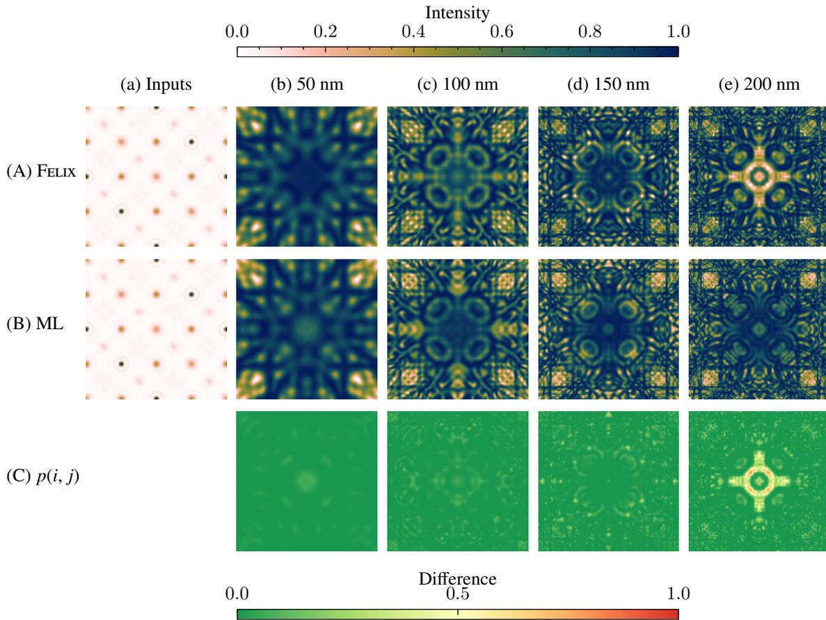
Figure 6: Differences in FELIX (row A) and cGAN (row B) bright field LACBED simulations for  $\text{Dy}_2\text{Ti}_{1.9}\text{O}_{6.95}$  (ICSD 249064,  $\text{Fd}\bar{3}mZ$ ), an example close to the mean performance for each thickness. Row C shows the pixel-by-pixel squared intensity differences (5); cross-correlations  $R$  are (a) 0.967, (b) 0.926, (c) 0.903, and (d) 0.766.
