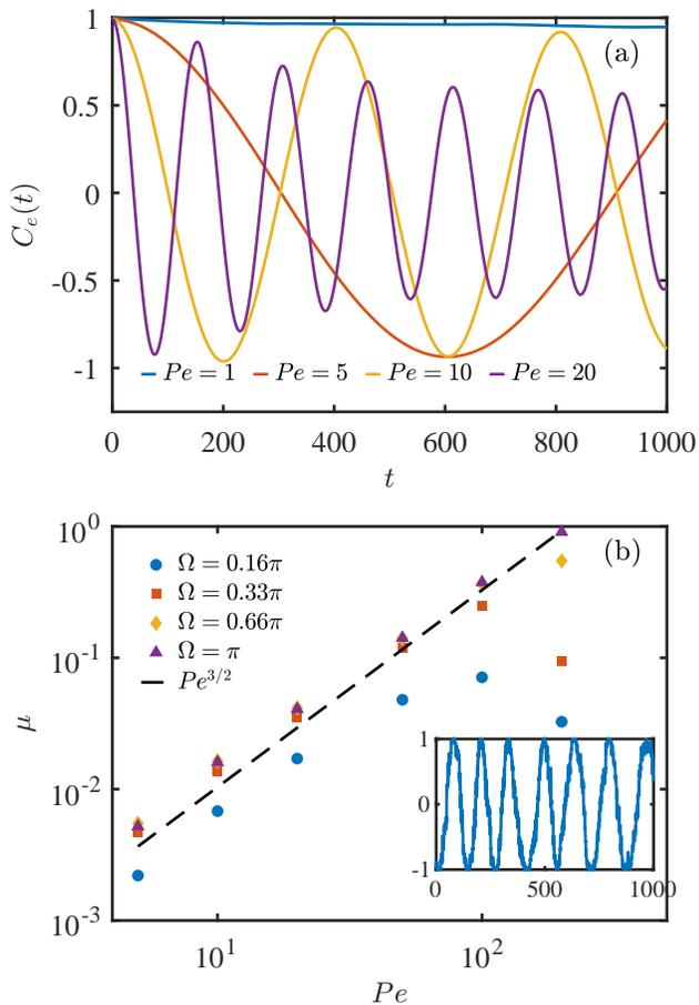
FIG. 10: a) End-to-end correlation at  $\Omega = \pi$ . b) Frequency of rotation as a function of  $Pe$ . Inset displays the time-series data of x-component of end-to-end vector at  $Pe = 20$  for  $\omega = 2\pi$ .
