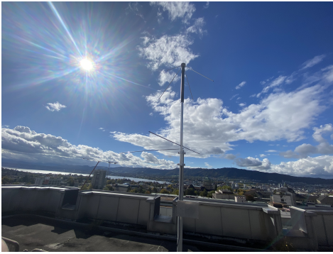
Fig. 2. Turnstile antenna for the data acquisition system deployed on a rooftop in Zurich.
