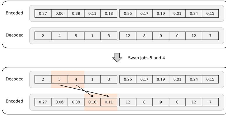
**Figure 7:** Local search on a single-machine example individual
