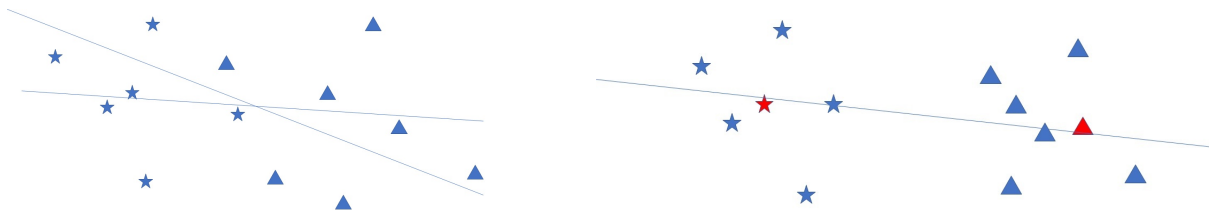
Fig. 1. Left: Reconstruction loss based autoencoder latent space is not optimized for regression. Right: Clustering in the latent space can improve regression due to the samples being more sparsely distributed (with respect to their cluster mean, as depicted in red).
