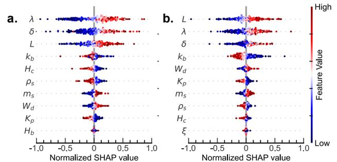
FIGURE 3. Feature importance by Shapley value against (a) the maximum column drift and (b) the maximum bearing displacement.
