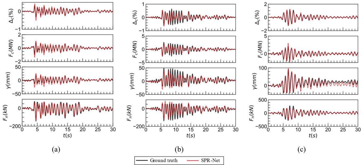
**Figure S5. Seismic response predictions of the deterministic SPR-Net model for column peak drifts at (a) 16<sup>th</sup>, (b) 50<sup>th</sup>, and (c) 84<sup>th</sup> CDF percentiles**
