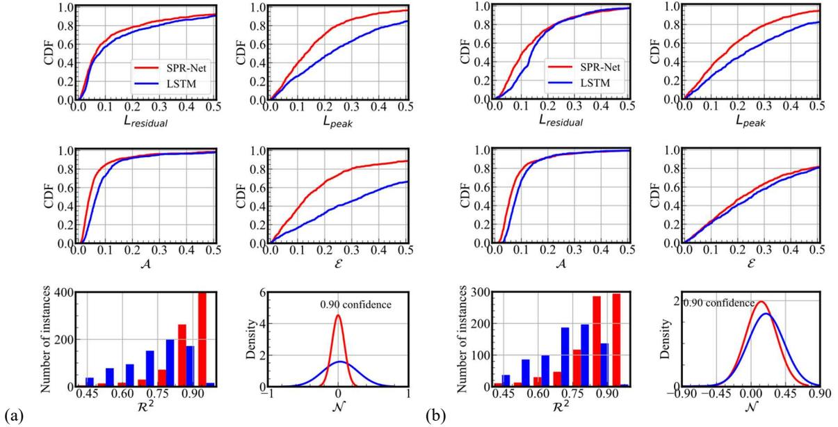
**Figure S7. Comparisons of the deterministic SPR-Net model and the LSTM model for (a) column drift and (b) the bearing displacement**
