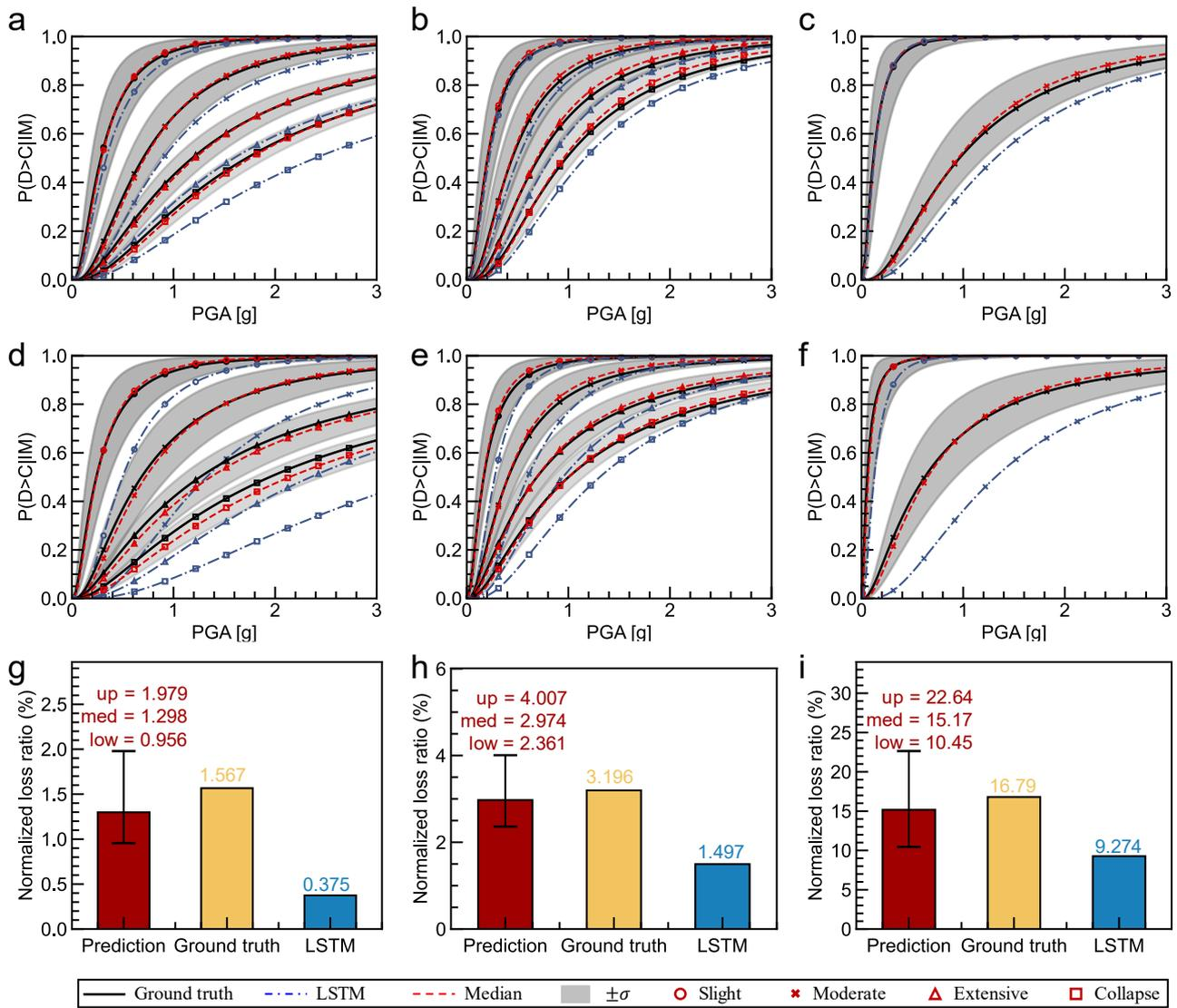
**FIGURE 6. Comparisons of seismic fragility curves and seismic loss estimations. Class fragility:** (a) column using drift ductility (b) column using the Park-Ang index (c) bearing using peak displacement; **Fragility for the soft bridge:** (d) column using drift ductility (e) column using the Park-Ang index (f) bearing using peak displacement (g) column loss ratio using drift ductility (h) column loss ratio using the Park-Ang index and (i) bearing loss ratio using peak displacement.
