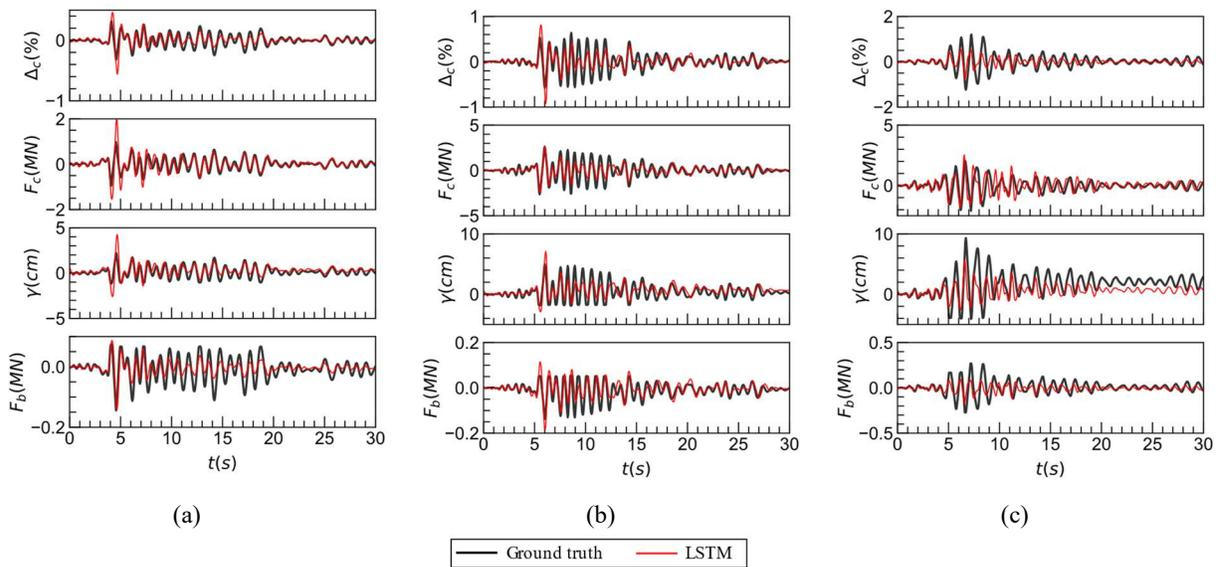
**Figure S6. Seismic response predictions of the LSTM model for column peak drifts at (a) 16<sup>th</sup>, (b) 50<sup>th</sup>, and (c) 84<sup>th</sup> CDF percentiles**
