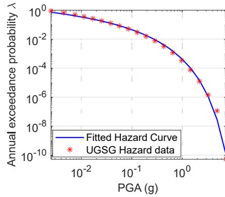
**Figure S9. Seismic hazard curve for the considered bridge site at Los Angeles**
