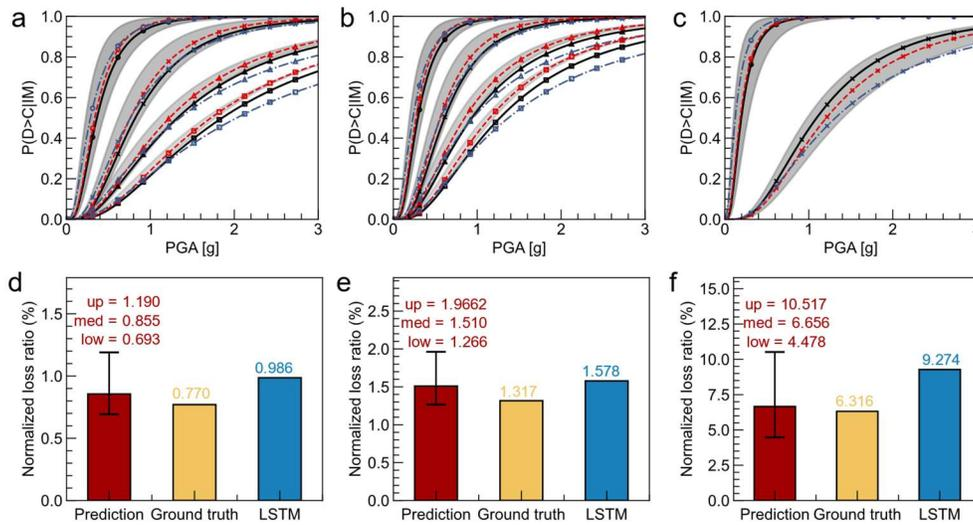
**Figure S11. Comparisons of seismic fragility curves and seismic loss estimations for the stiff bridge. (a) column fragility using drift ductility (b) column fragility using the Park-Ang index (c) bearing fragility (d) column loss ratio using drift ductility (e) column loss ratio using Park-Ang index and (f) bearing loss ratio.**
