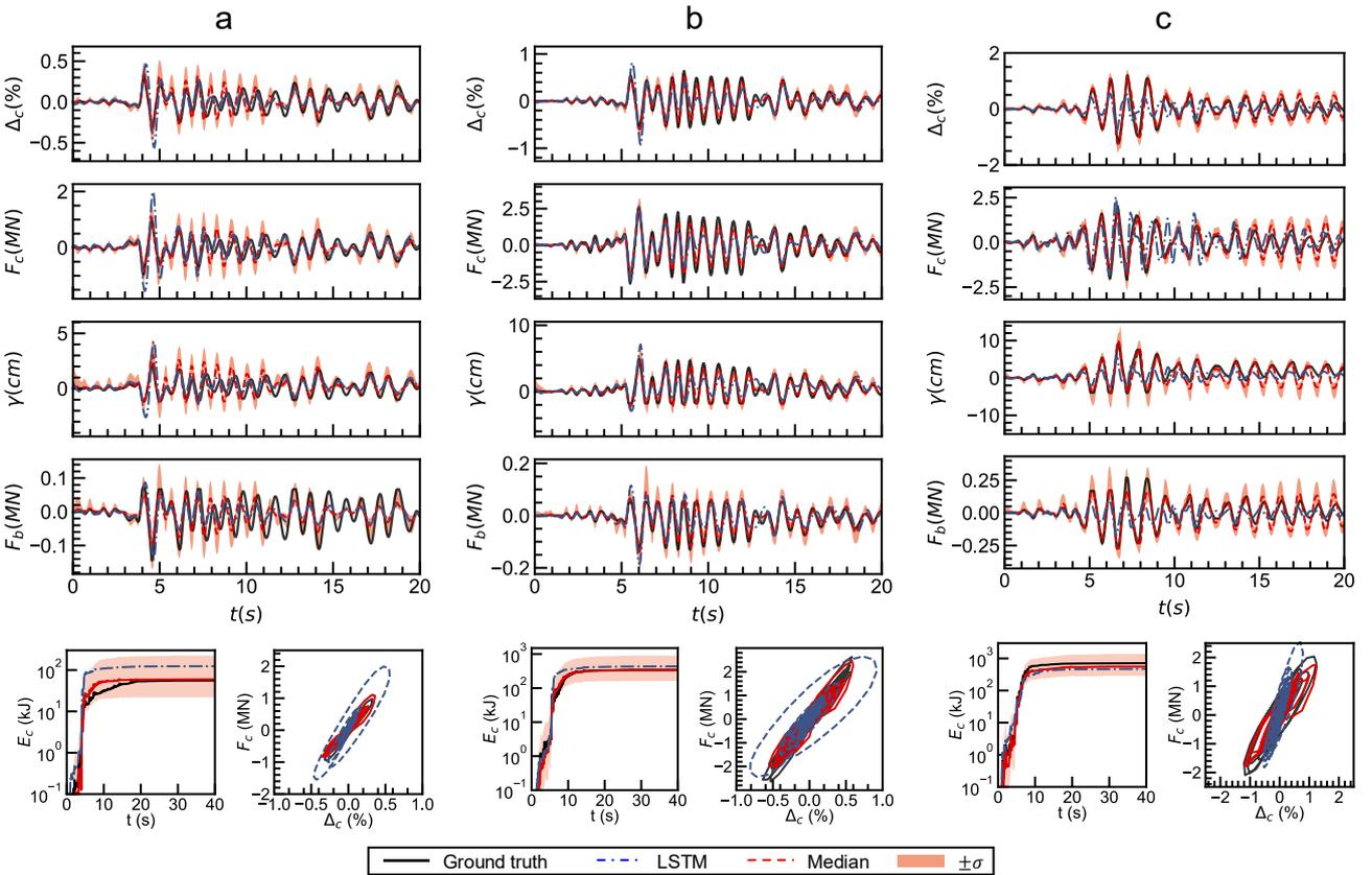
**FIGURE 5.** Time series response comparisons for column drift ratios at (a) 16<sup>th</sup>, (b) 50<sup>th</sup>, and (c) 84<sup>th</sup> CDF percentiles.
