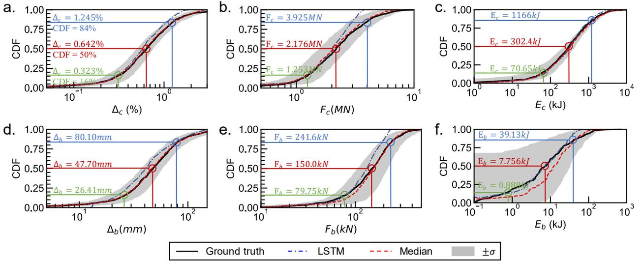
**FIGURE 4.** CDF comparisons of different response metrics from LSTM and SPR-Net. (a) peak column drift ratio, (b) peak column lateral force, (c) dissipated energy of column, (d) peak bearing displacement, (e) peak bearing lateral force, and (f) dissipated energy of bearing. 16<sup>th</sup>, 50<sup>th</sup> and 84<sup>th</sup> percentile CDF values are listed in each figure.
