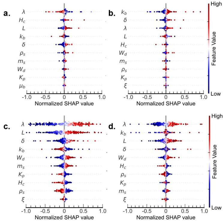
**Figure S8. Shapley values of bridge parameters for (a) column energy dissipation, (b) bearing energy dissipation, (c) enclosed area of column deformation, and (d) enclosed area under bearing deformation**
