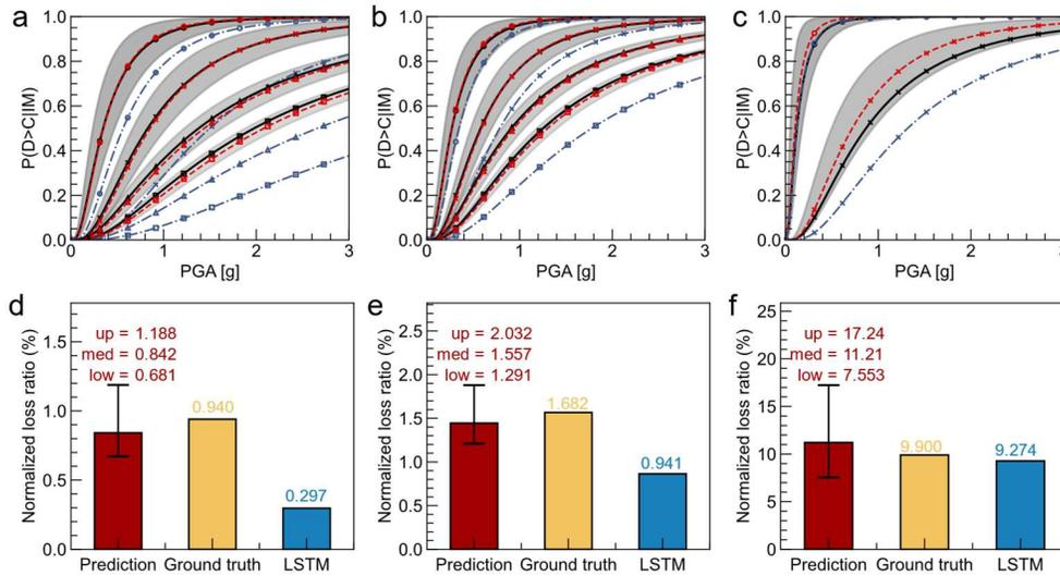
**Figure S10. Comparisons of seismic fragility curves and seismic loss estimations for the medium bridge. (a) column fragility using drift ductility (b) column fragility using the Park-Ang index (c) bearing fragility (d) column loss ratio using drift ductility (e) column loss ratio using Park-Ang index and (f) bearing loss ratio.**
