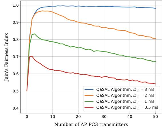
Fig. 7. JFI among Wi-Fi and NR-U networks with QaSAL algorithm for various delay thresholds and varying number of PC3 transmitters.
