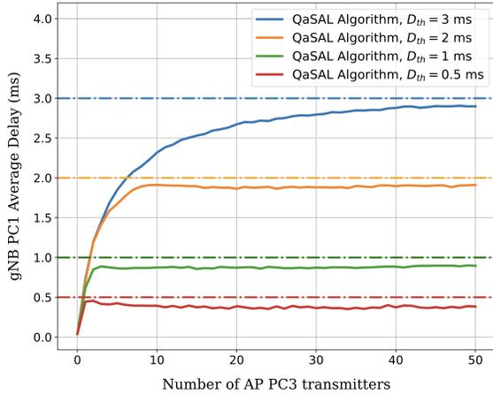
Fig. 6. Average Transmission delay of PC1 transmitter with QaSAL algorithm for various delay thresholds and varying number of PC3 transmitters.
