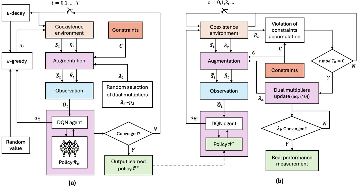
Fig. 2. The flowchart of QaSAL algorithm for CPM: a) Training phase b) Execution phase.
