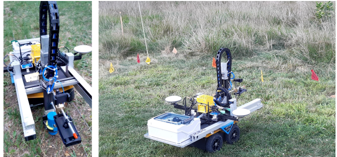
Fig. 2: left ) view of the 3-D mechanical arm and Holographic Subsurface Radar (HSR); right ) a panoramic view of the Robotic platform. This system has been used to acquire the basic elements used to create the dataset.
