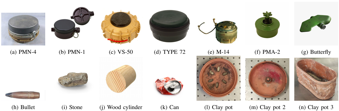
Fig. 5: Objects considered for indoor scans. On the first row, landmines replicas are reported, namely (from left to right): PMN-4 ( d=95\text{mm} , h=46\text{mm} ), PMN-1 ( d=95\text{mm} , h=55\text{mm} ), VS-50 ( d=90\text{mm} , h=45\text{mm} ), TYPE 72 ( d=78\text{mm} , h=38\text{mm} ), M-14 ( d=56\text{mm} , h=40\text{mm} ), PMA-2 ( d=68\text{mm} , h=61\text{mm} ), and Butterfly ( l_1=112\text{mm} , l_2=60\text{mm} , h=15\text{mm} ). The second row shows the Bullet ( d=20\text{mm} , l=120\text{mm} ), some clutter (stone ( l_1=110\text{mm} , l_2=56\text{mm} , h=34\text{mm} ), wood cylinder ( d=35\text{mm} , h=40\text{mm} ), and crumpled can ( l_1=110\text{mm} , l_2=62\text{mm} , h=15\text{mm} ), and some pottery objects (perforated clay pot ( d=180\text{mm} , h=28\text{mm} ), clay pot ( d=170\text{mm} , h=24\text{mm} ), and deep clay pot ( l_1=120\text{mm} , l_2=265\text{mm} , h=135\text{mm} )).
